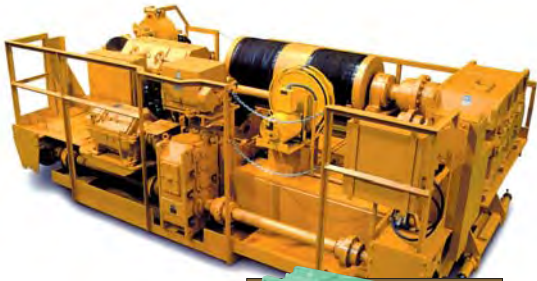
Sumitomo Paramax® reducers provide quiet, reliable operation for both the hoist and trolley drive systems in this 35-ton capacity DC Trolley Hoist used for heavy-duty coil handling service.
