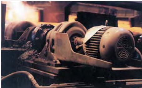
After molten steel is formed in the five-strand continuous caster at this steel mill, it is conveyed by Sumitomo Cyclo® drives on the auto-torch conveyors where the steel is cut into billets.
