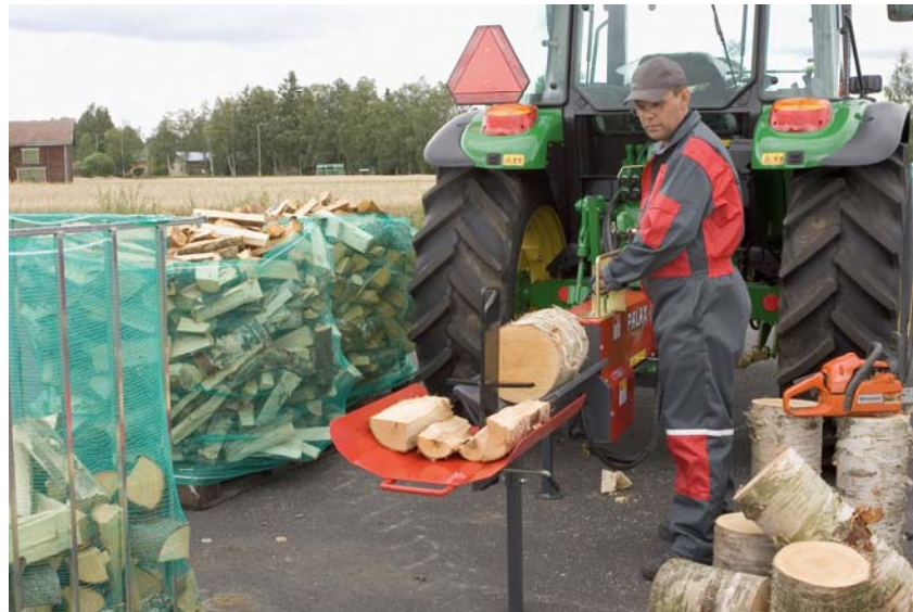
Figure 10. Tractor-driven hydraulic splitter. Photo: Terästakomo Oy.
