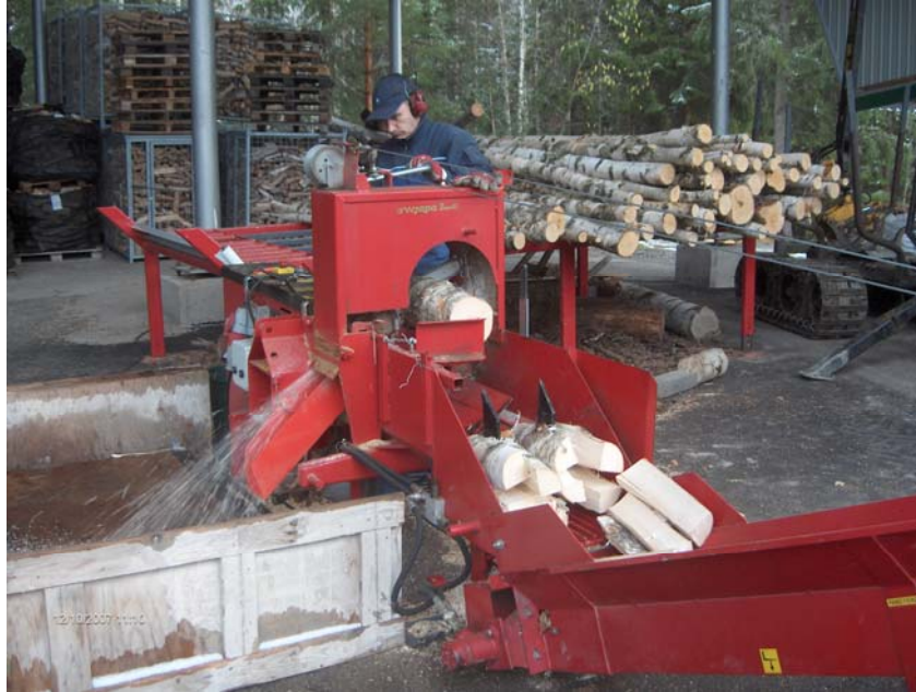
Figure 11. A two-stage chopping machine that saws and splits the wood. Photo: Ari Erkkilä, VTT.
