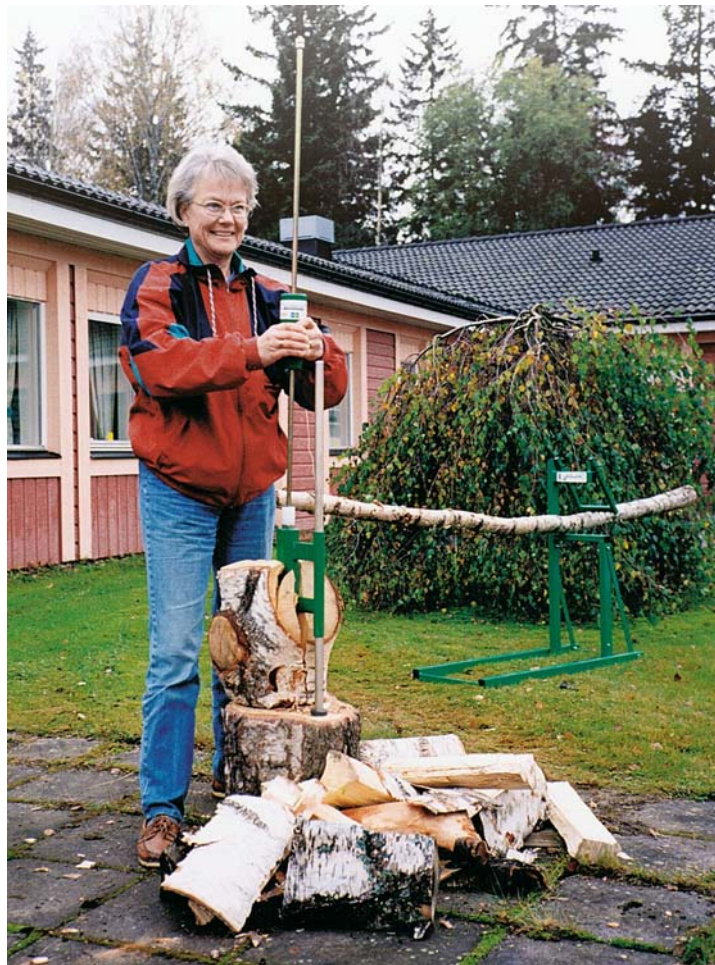
Figure 7. The Smart Splitter controls the force of impact against the wedge. Photo: Oscar trade.
