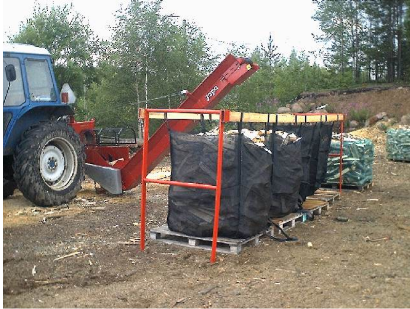
Figure 12. These chopped logs are being stored in breathable sacks where they will dry. Machine power is needed to deposit the logs. Photo: Isto Mäkelä.
