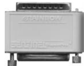
Figure 10: D6201 Parallel Port Security Key
