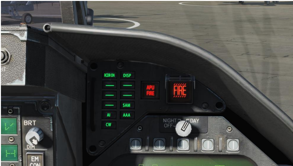
Figure 91. Right Instrument Panel Warning / Advisory / Threat Display Panel
