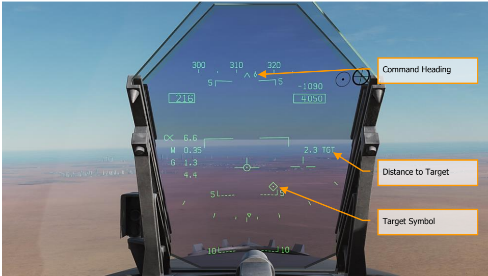
Figure 40. Waypoint as Target on HUD
