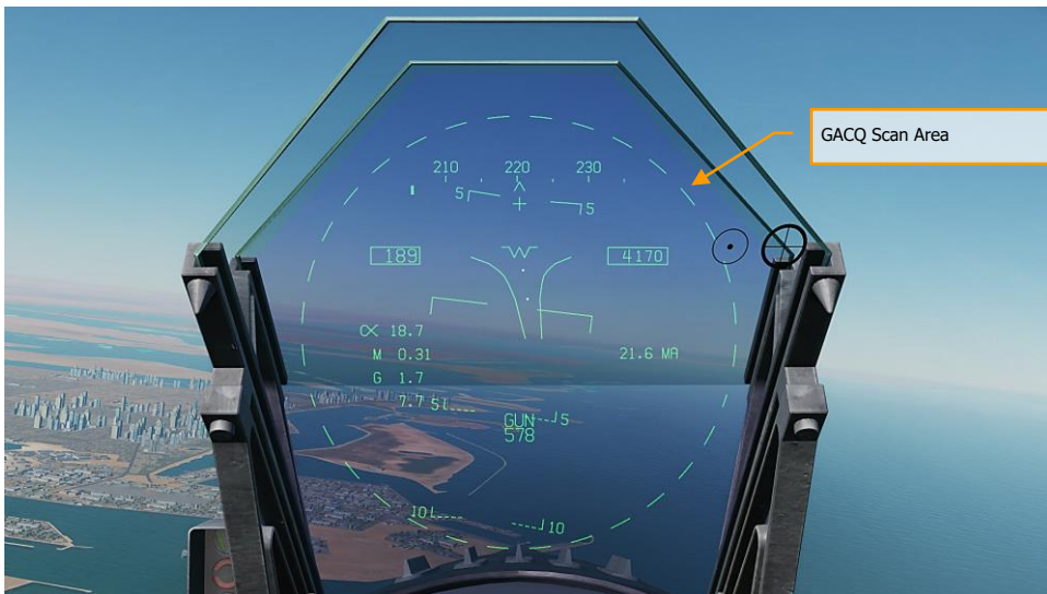
Figure 70. A/A GUNS Auto Acquisition Area
