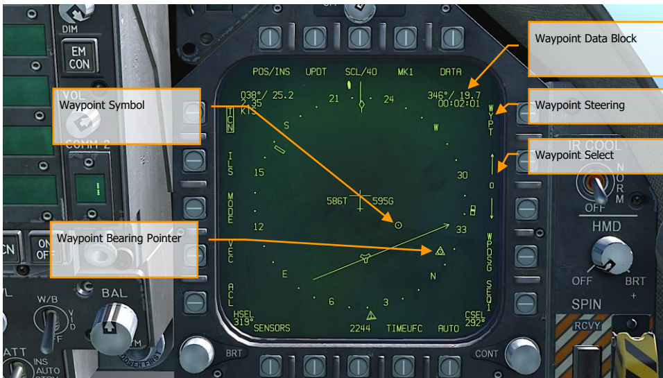
Figure 38. HSI Waypoint Steering
