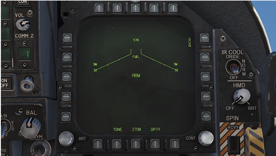
Figure 31. Stores Management System (SMS) Page
