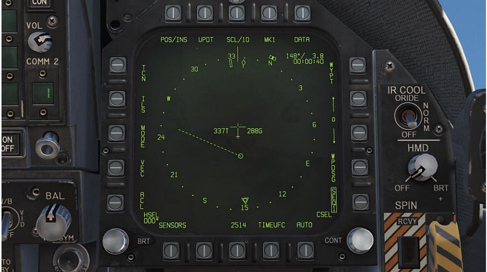
Figure 26. Horizontal Situation Indicator (HSI) Page
