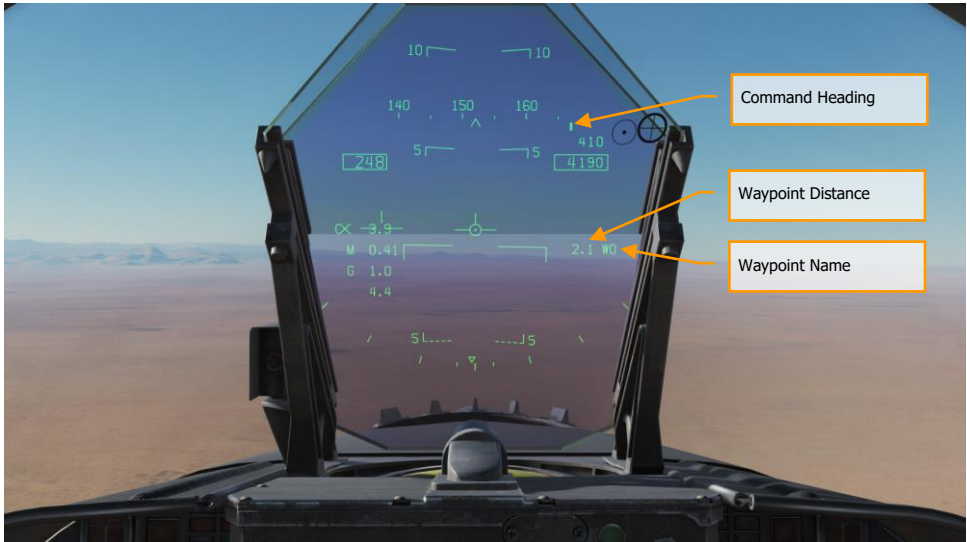
Figure 39. Waypoint Steering on HUD
