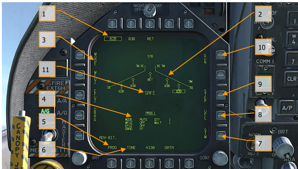
Figure 51. A/G Conventional Bombing SMS Page
