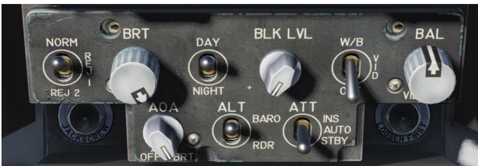
Figure 11. HUD Control Panel
