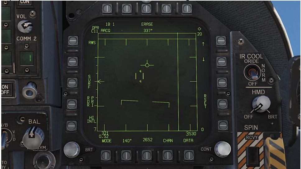
Figure 30. Attack RADAR Page
