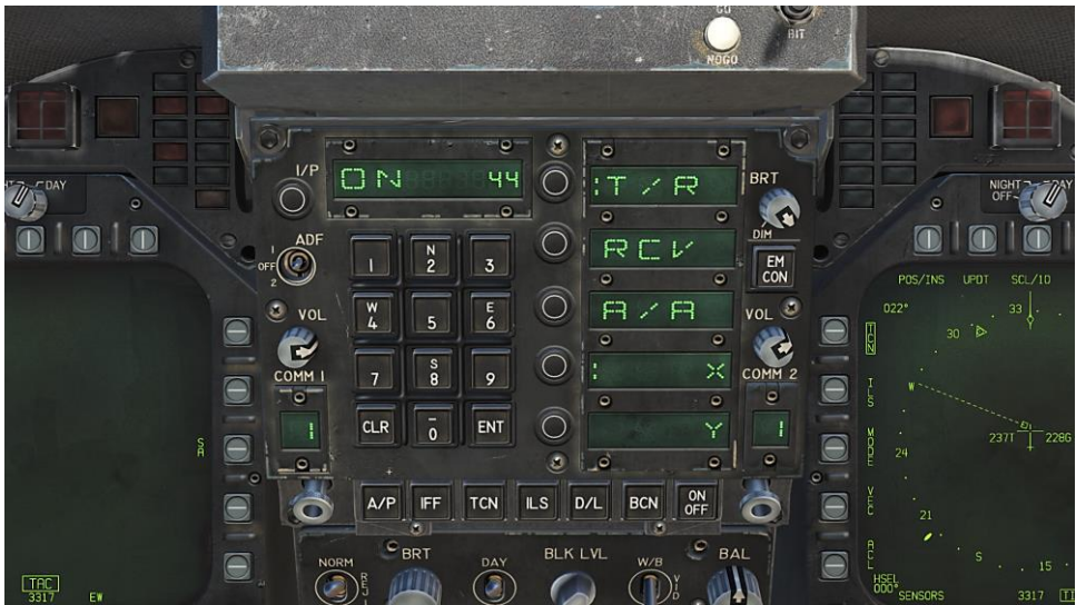
Figure 41. TACAN Options on UFC
