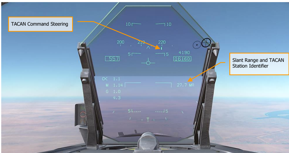
Figure 43. TACAN Steering on HUD
