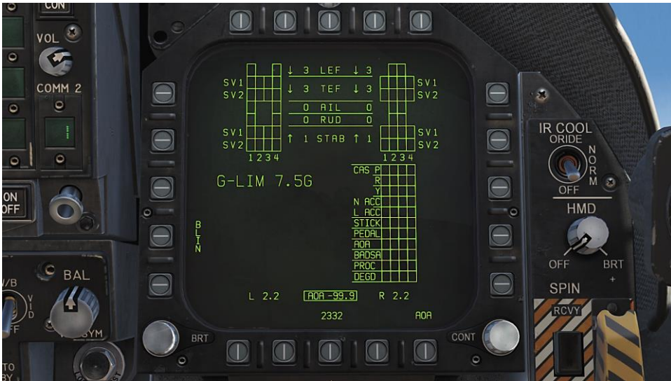
Figure 23. Flight Control System (FCS) Page
