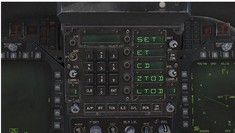
Figure 37. TIMEUFC Options on UFC
