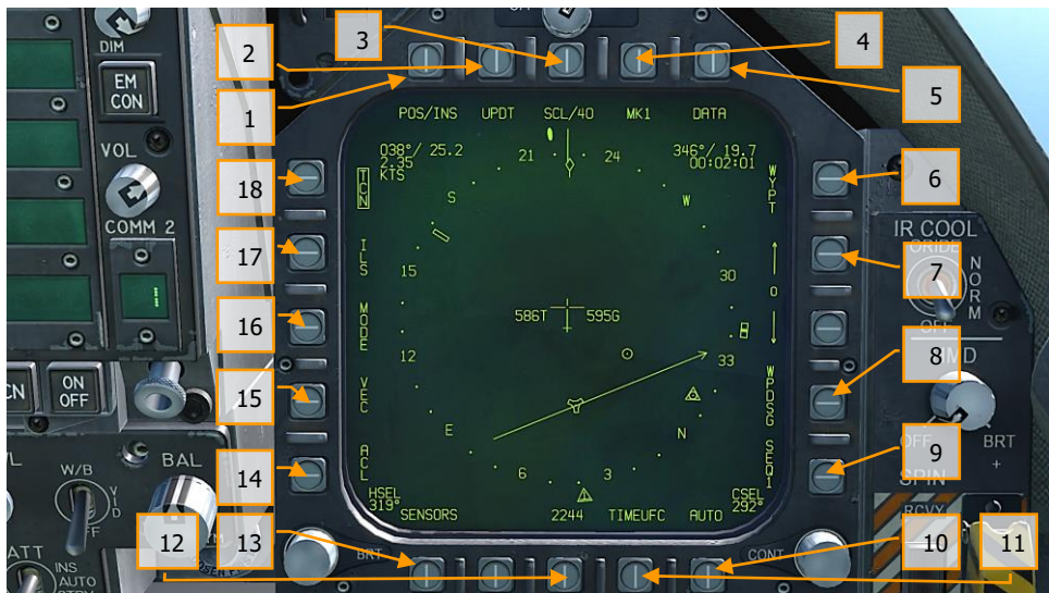
Figure 35. HSI Option Buttons
