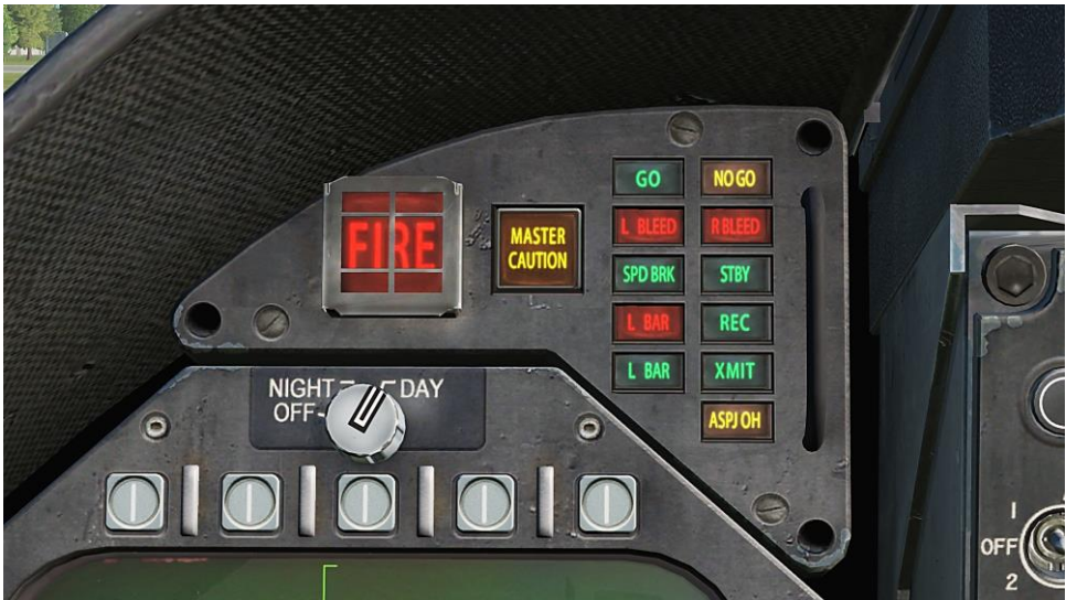
Figure 85. ASPJ annunciator panel
