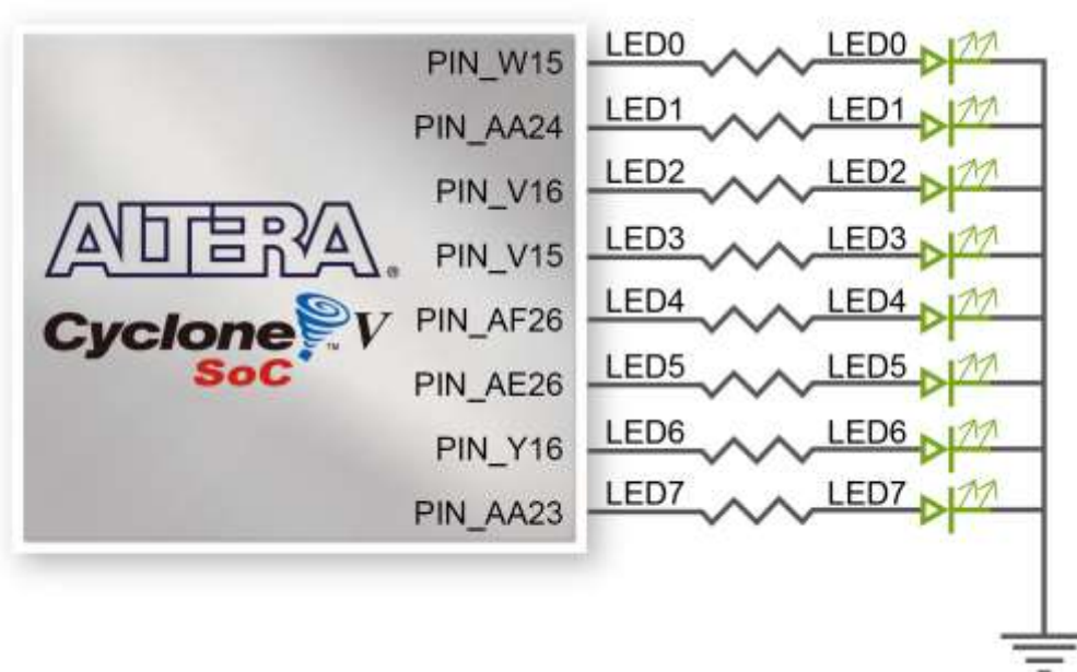
Figure 3-19 Connections between the LEDs and the Cyclone V SoC FPGA
