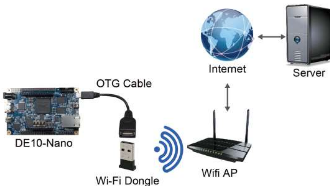
Figure 6-9 System diagram of USB Wi-Fi dongle
