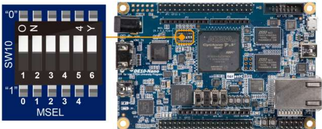
Figure 3-1 DIP switch (SW10) setting of FPPx32 mode.
