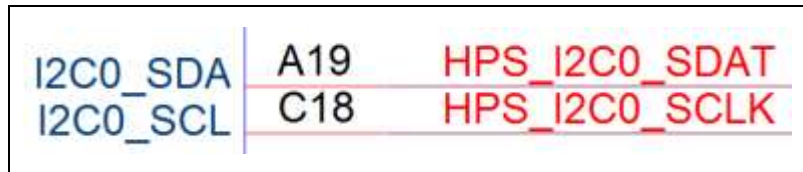
Figure 6-7 Connection of HPS I2C signals
