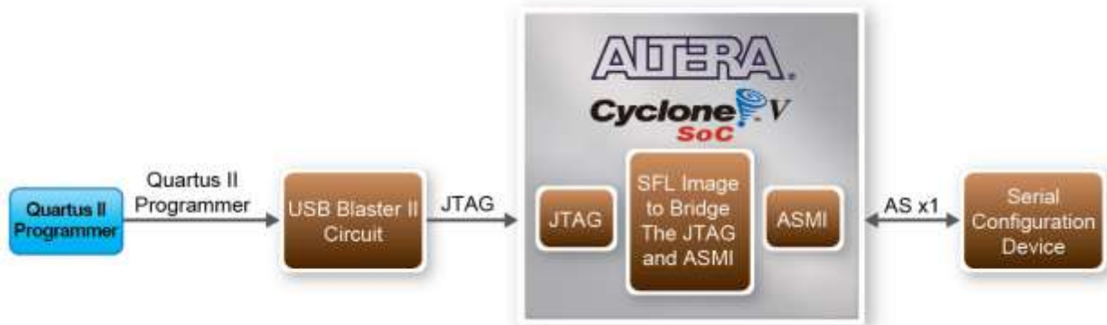
Figure 3-11 Programming a serial configuration device with SFL solution
