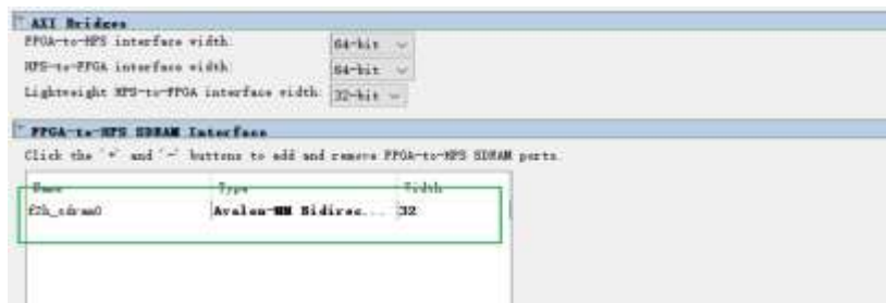
Figure 5-19 F2H SDRAM Interface Setting
