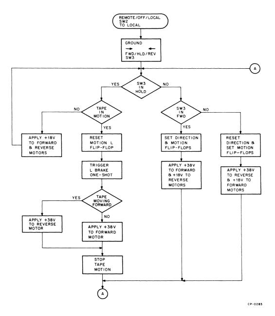
Figure 3-4 Off-Line Manual Operation Flow Chart
