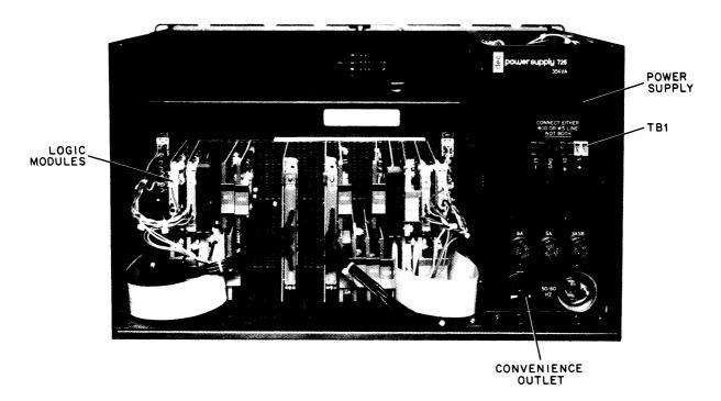
Figure 1-3 Power Supply Location
