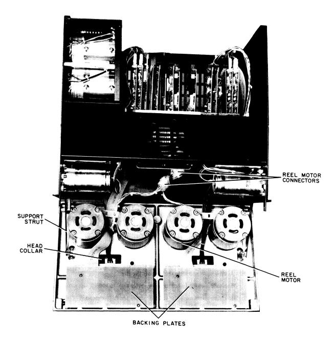
Figure 4-1 Reel Motor Removal
