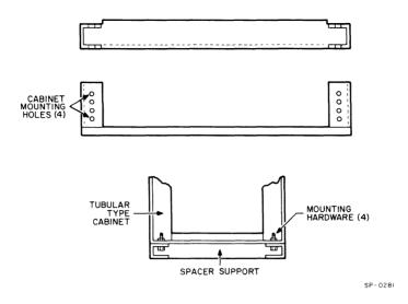
Figure 2-4 Tubular Cabinet Spacer Support Bracket
