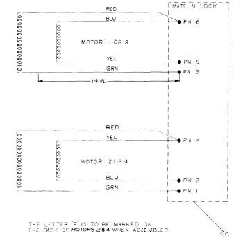
MOTOR WIRING DIAGRAM
