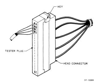
Figure 4-4 Skew Tester to Head Cable Connection
