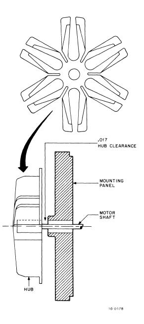
Figure 4-2 Reel Hub Clearance
