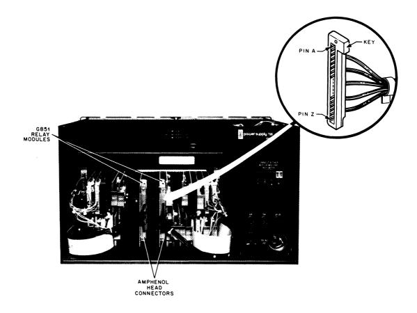
Figure 4-3 Head Connector Location
