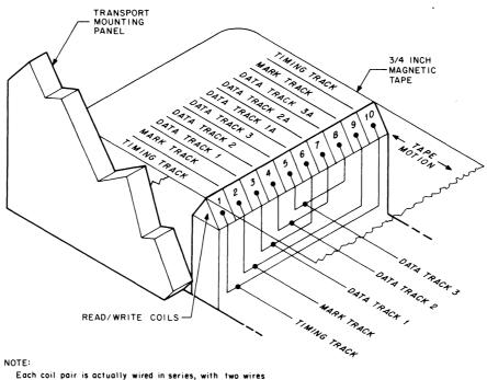
connected to a differential amplifier. However, for simplicity, only a single wire from each pair is shown.
