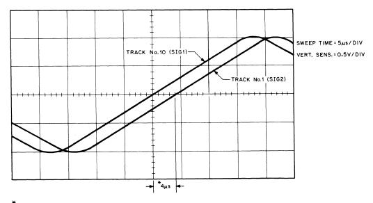
Zero crossing time equals twice the skew time. Actual skew = 2,µs. For best transport operation, head skew should be as close to zero as possible.
