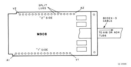
Figure 4-7 M908 Module Layout
