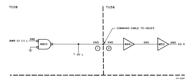
Figure 3-1 TC08 to TU56 Logic Connection
