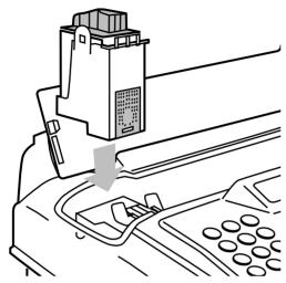
• Push the cartridge towards the front of the machine until it clicks into place.
