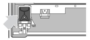
To remove the print head, pull back the two green tabs to release the catch and lift the cartridge out.
