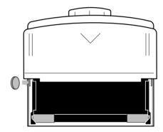
Insert a small coin in the groove at the bottom of the automatic sheet feeder to release the black side supports.
