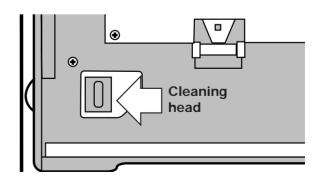
When the printer cover is opened, the ink cartridge automatically moves to the centre of the machine. However, if your DF450 is not connected to the mains, you can move the printer head by gently pushing it along its runner to reveal the print cartridge cleaning head.
