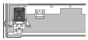
The ink cartridge is located inside the print head. The print head does not need to be removed while changing the ink cartridge.
