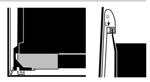
Replace the paper cover on the front of the automatic sheet feeder.
