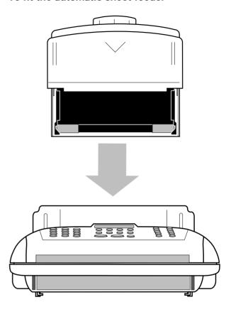
• Slot the automatic sheet feeder cassette into the main unit. Make sure it is fully inserted.
