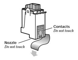
Avoid touching the print nozzle or the electrical contacts, as this may damage the print cartridge.
