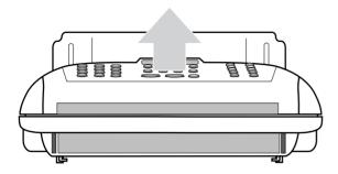
Release the green lever on the left-hand side of the white roller. Lift out the white roller.
