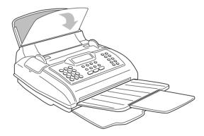
Remove the jammed sheet and close the cover. You may need to remove the whole paper tray.
