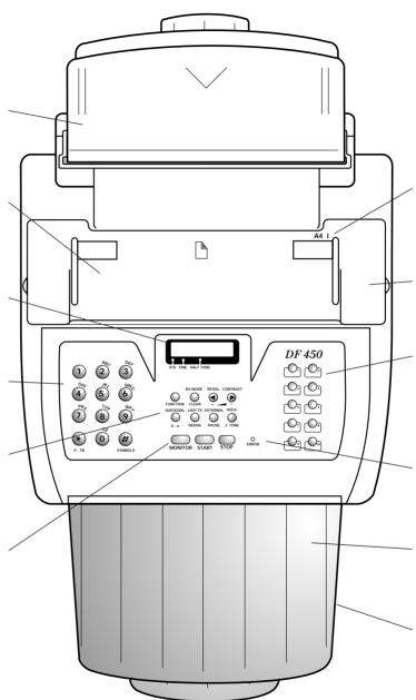
Adjustable paper guide. Place documents face down to ensure straight feeding into the machine for fax transmission.
