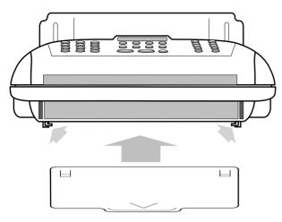
• Slide the received document tray into the slots on the base of the main unit.
