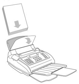
When adding more paper before the feeder is empty, load the new paper behind the existing pages in the cassette.
