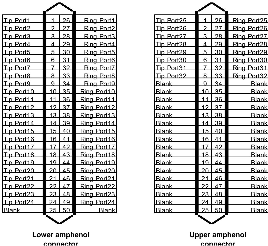
Figure 4.5.11-2 SLTM32 RJ-21X Connector Configuration
