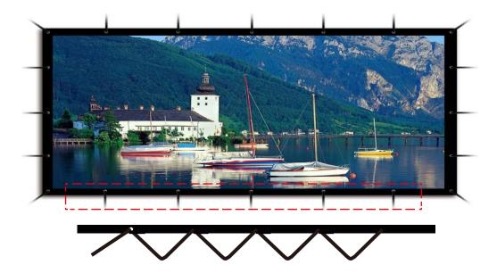
Tightly fasten the Polypropylene rope throughout each grommet to make the screen flat while fastening the rope to the installation location. Do several tests to ensure the rope stretches the material to its maximum extent. Once the approximate length of rope that is needed can be determined, remove any excess rope by simply cutting it.
