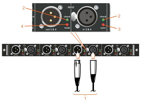
**1** Four pairs of digital **AES3** (AES/EBU) XLR inputs and outputs.
