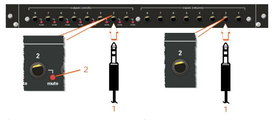
1 Eight jack sockets per **inputs (returns)** section and eight jack sockets per **outputs** (sends) section.
