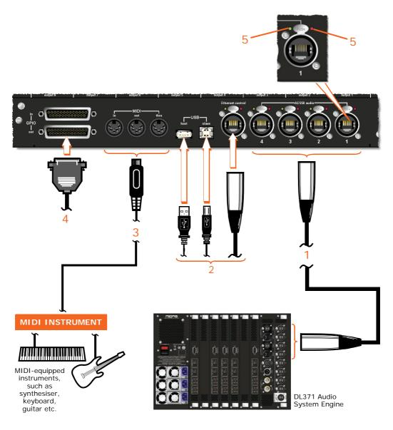
**1** Four **AES50 audio** Ethernet sockets for passing audio and control data to/from the DL371 Audio System Engine.
