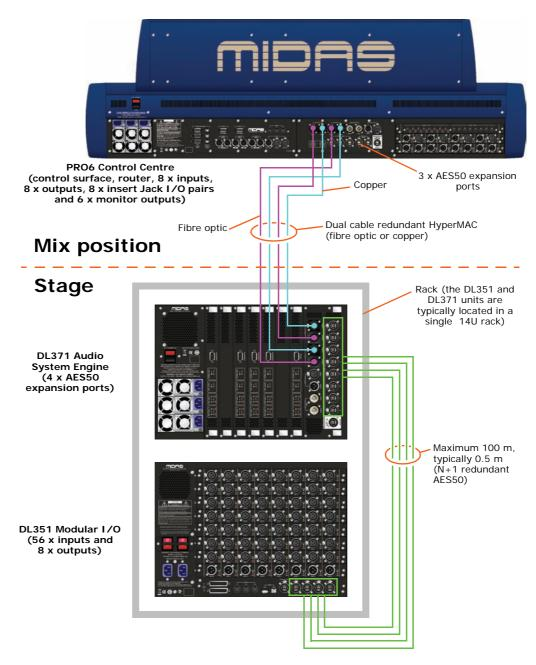
Figure 2: Standard system configuration
