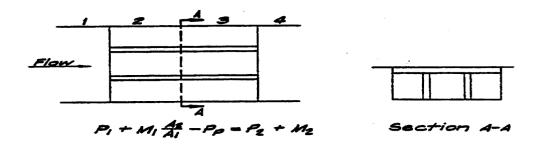
where  $P_1$  = Hydrostatic pressure in unobstructed channel
