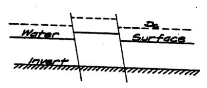
(d) If, at the upstream end of the pier, no depth can be found to balance the P+M equation, calculate P+M for the depth of flow just outside the upstream end of the pier and its sequent depth. If the lower stage results in the greater sum (P+M), this indicates a hydraulic jump at the upstream face of the pier. If the upper stage results in the greater sum (P+M), this indicates a hydraulic jump some distance
