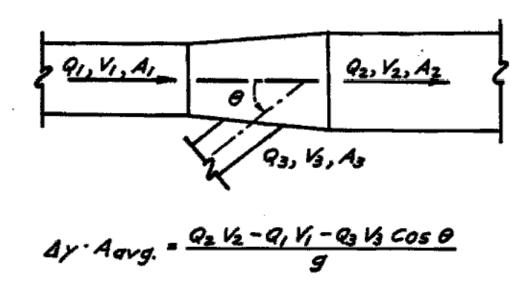
Where  $\Delta y =$  difference in hydraulic gradient for the two end sections, in feet  $A_{avg} =$  average area, in feet<sup>2</sup> = 1/6 ( $A_1 + 4A_m + A_2$ ) or, for practical use 1/2 ( $A_1 + A_2$ )  $A_m =$  mean area of flow, in feet<sup>2</sup>
