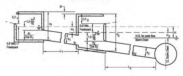
Select a connector pipe size for each storm inlet, and determine the related head loss ( $H_1$ ,  $H_2$ ) by means of a culvert equation, or by Plate 22.3 D-9. The sum of head losses in the series should not exceed the available head, i.e.,
