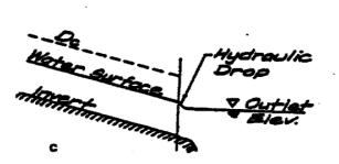
(c) Where the water surface of the outlet is below the water surface in the channel or conduit, control is upstream and the outflow will have the form of a hydraulic drop.
