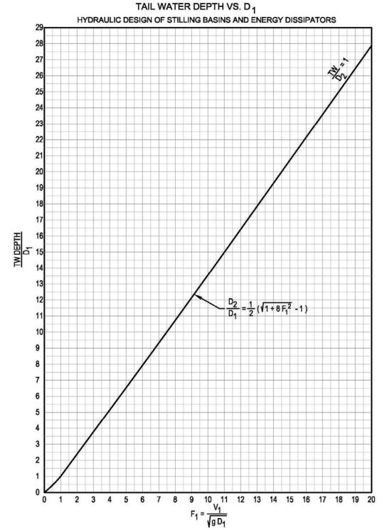
PLATE 22.3 E-1 FIGURE5. - RATIO OF TAIL WATER DEPTH TO D<sub>1</sub> (BASIN I)
