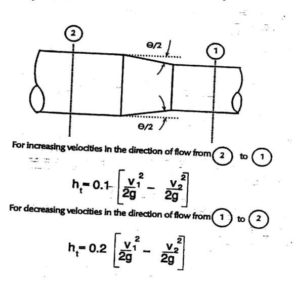
Deviations from the above criteria must be approved by the City Engineer/SSCAFCA. When such situations occur, the angle of divergence or convergence ( $\theta$ /2) may be greater than 5 degrees 45 minutes. However, when it is increased beyond 5 degrees 45 minutes, the above equation will give results for  $h_t$  that are too small, and the use of more accurate methods, such as the Gibson method shown Plate 22.3 B-2, will be acceptable.
