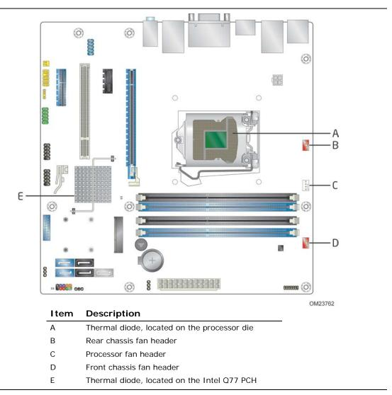
Figure 6. Thermal Sensors and Fan Headers
