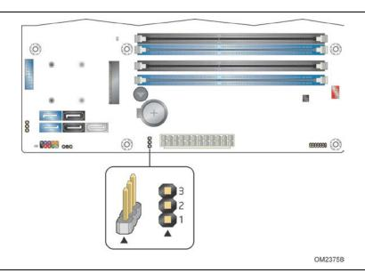
Figure 15. Intel MEBX Reset Header
