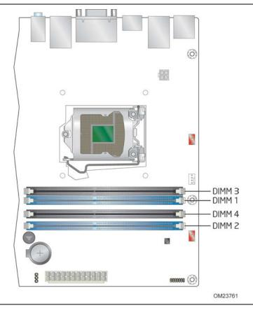
Figure 3. Memory Channel and DIMM Configuration
