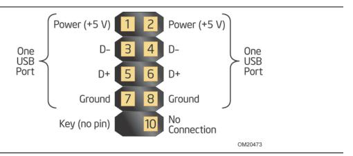
Figure 13. Connection Diagram for Front Panel USB 2.0 Connectors
