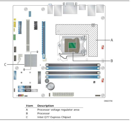
Figure 17. Localized High Temperature Zones
