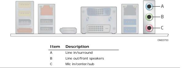
Figure 4. Back Panel Audio Connectors
