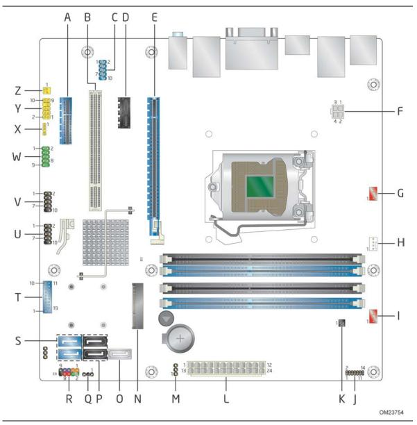
Figure 11. Component-side Connectors and Headers
