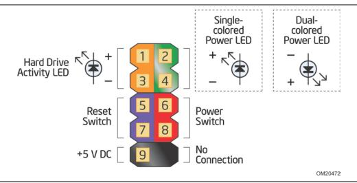
Figure 12. Connection Diagram for Front Panel Header
