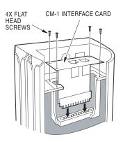
Figure 5.2.6 CM-1 Interface Card (See Installation Instructions with Card)
