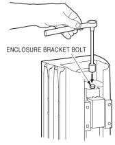
Figure 5.6.9d Secure the Enclosure Position
