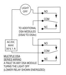
Annunciator OFF for a fault condition: Connect to the NO and COM terminals. The terminals are wired in series to each module.
