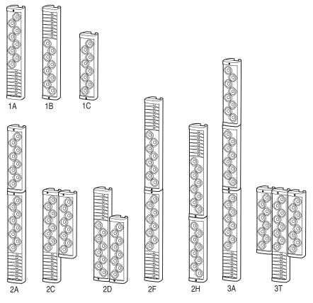
Figure 5.6.3 DSAi Cluster Configurations
