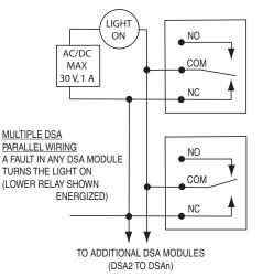
Figure 5.3.3c Multiple DSAi Fault ON
