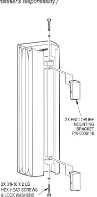
Figure 5.6.8 Enclosure Bracket Installation
