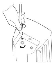
Figure 5.4.3 Connecting AC Mains
