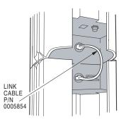
Figure 3.4a Signal Links < 1 ft / 0.3 m
