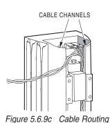
3. Route cabling as required using the rear channels in the enclosure's extrusion.
