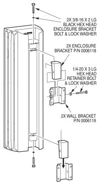
Figure 3.6.2a Bracket Installation
