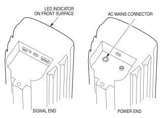
Figure 3.6 Signal End / Power End
