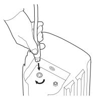
Figure 3.5 Connecting AC Mains
