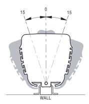
Figure 5.6.5a Horizontal Rotation Single Module
