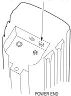
FAULT DETECT RELAY CONNECTOR
