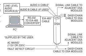
Figure 5.1 Electrical Block Diagram
