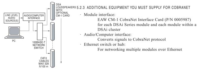
Figure 5.2.3 Basic CobraNet Diagram
