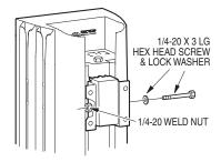
Figure 5.6.9b Retainer Bolt Installation
