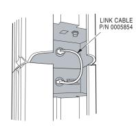
Figure 5.1.4 Linking < 1 ft / 0.3 m
