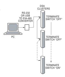
Figure 5.1.6b EIA-485 Network Diagram
