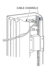
Figure 5.1.1 Cable Channels
