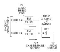
Figure 5.5.2b Ground Lift Function
