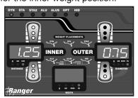
5. Attach the specified weight for the appropriate **PLANE** position at top-dead-center.
