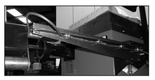
6. Attach the end of the wire to the connection on the back side of the balancer.
