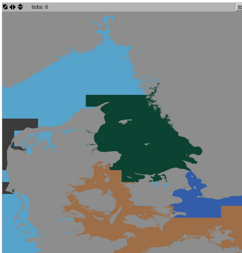
Figure 12. Hydrographic regions displayed in the World View following the termination of the cluster analysis. This example show 4 regions with unique colors.
