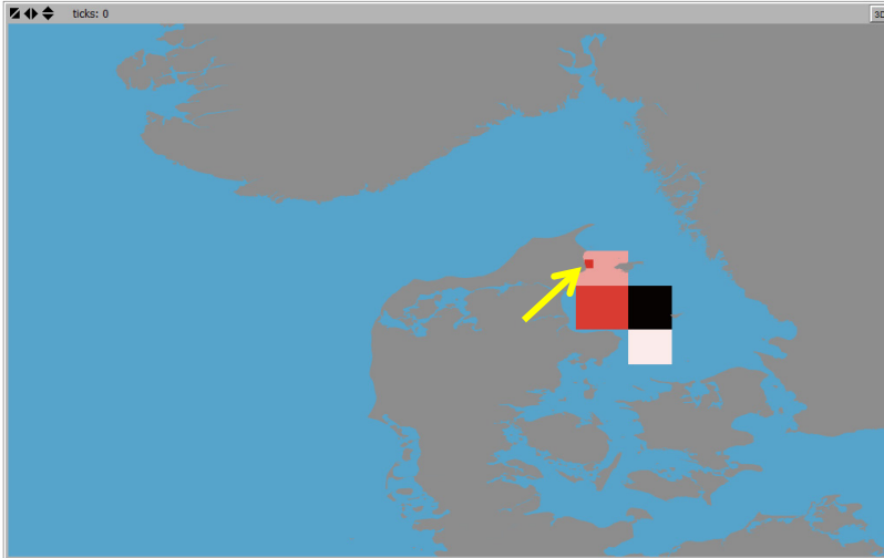
Figure 18. Upstream connectivity probability of a specified location indicated by yellow arrow. The color legend range from 0 (blue) to 0.356 (darkest red). Values represent the probability that an agent with an end position in the specified location (grid cell indicated by a yellow arrow) will originate from (~have their start position in) any other grid cell.
