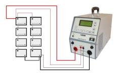
Otherwise, the charger keeps charging under the selected constant voltage, the current will decrease over time until it reaches a predetermined minimum value. At this point of time the charger will switch to a float charge stage and decrease to a selected float voltage.
