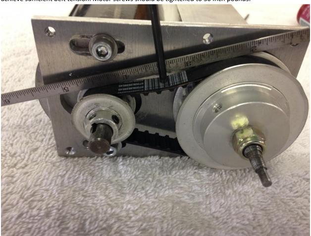
7. Replace the top and side plates of the drive enclosure using the 6 #8 screws removed in step 1. Start all 6 scews then tighten in two steps criscross pattern. Pulley swap is complete.
