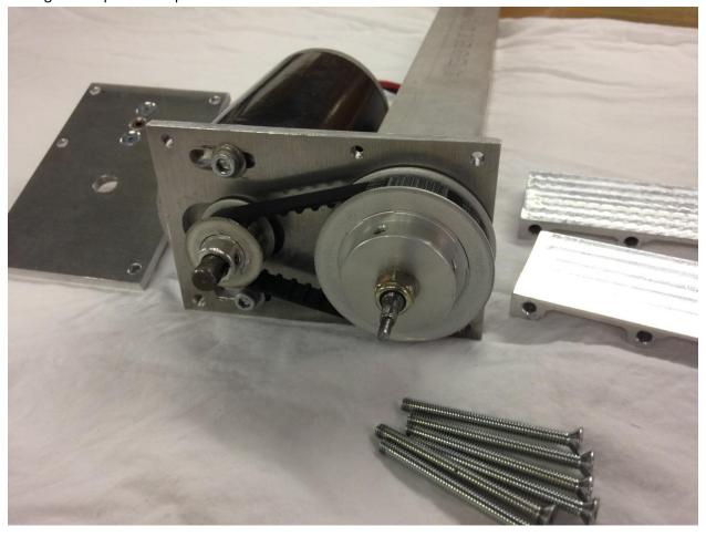
2. Loosen, but do not remove, the two #10 socket head cap screws securing the motor to the motor plate. Slide the motor toward the actuator housing such that the belt can be removed.
