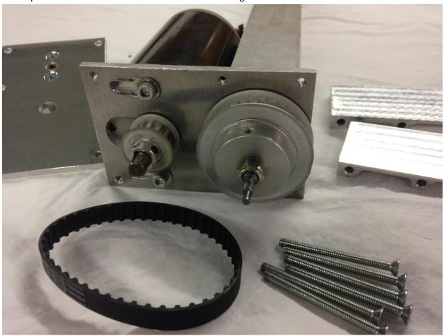
3. Remove the 5/16-24 Nylock nut securing the driven 30 tooth pulley to the lead screw. Using 2 flat blade screw drivers, carefully pry the pulley off the lead screw shaft as shown. Be careful not to lose the 2mmx10mm machine key captured between the pulley and shaft. Do not remove the
