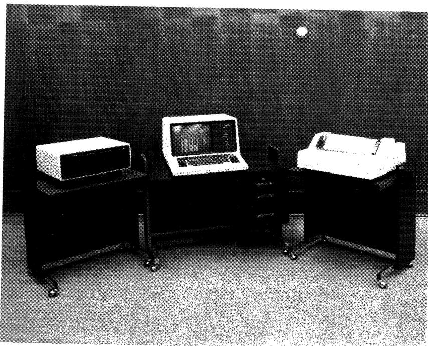
*This UTS 400 system includes the Master Station in the middle with display/keyboard, the standard dual diskette drive on the left, and the 200 cps 0786 matrix printer on the right.*
