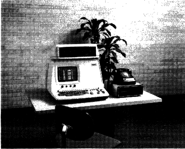
The PCS-II shown above has an independent processor to handle the communications line; two Minidiskette Drives sit atop the display unit. The compact system can function as a terminal or as a data processor.
