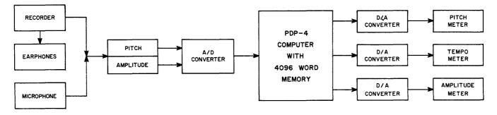
The Project SAID teaching machine includes an analog-todigital converter, general-purpose Programmed Data Pro-
