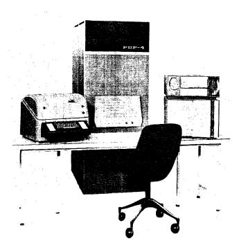
The PDP-4 is an 18-bit computer designed for scientific, engineering, and process control applications. It performs 1's or 2's complement binary arithmetic at a rate of 62,500 additions per second. Core memory, ranging from 1024 to 32,768 words, cycles in 8 microseconds, giving it an input/output transfer rate of 125,000 words per second.
