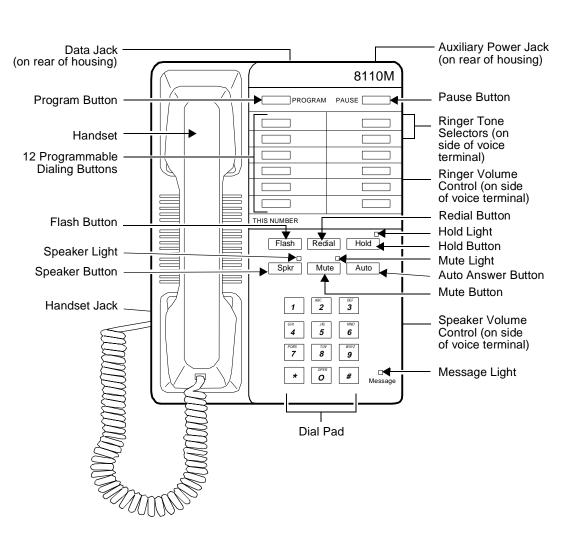
Figure 15-4. The 8110 and 8110M Telephones (The 8110M is shown here)
