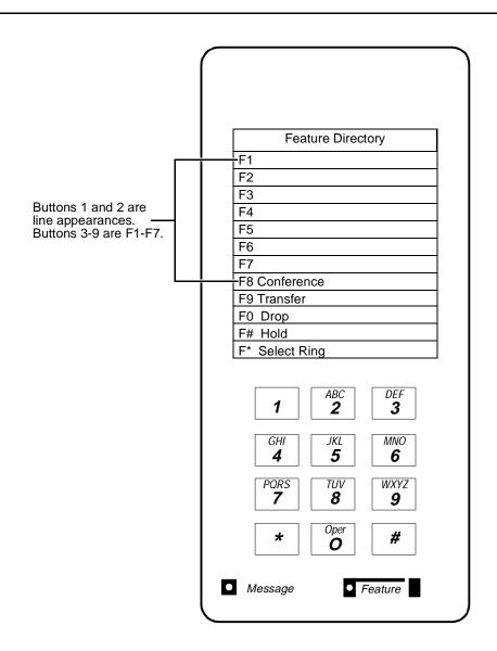
Figure 11-2. Button Number for Administering the 7401D and 7401 Plus Voice Terminals Connected to a System 75, DEFINITY G1 and G3, or a DEFINITY ECS
