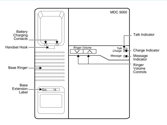
Figure 17-2. The MDC 9000 Telephone, Top View of Charging Base
