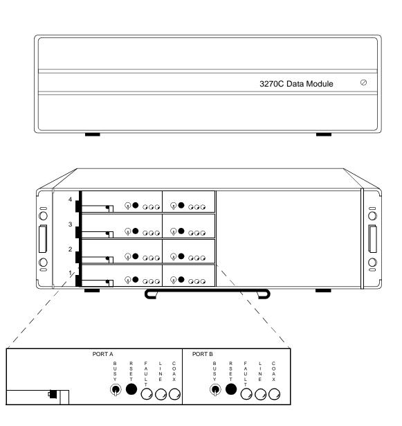
Figure 20-24. The 3270C Data Module
