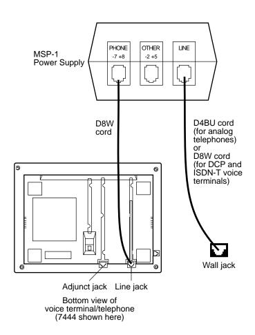
Figure 5-2. Local Powering Arrangement for: ISDN-T Voice Terminals; the DCP 7444 and 8434/8434DX Voice Terminals (for their VF Displays); and Adjuncts Connected to All Telephones Except the 8102
