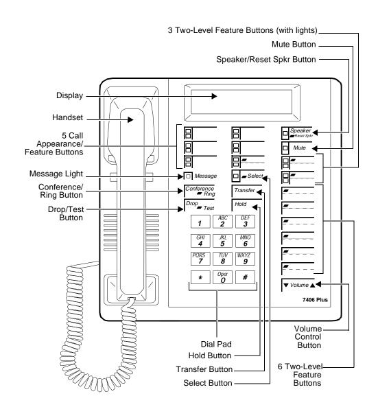
Figure 11-12. The 7406 Plus (7406D07A) Voice Terminal with Display
