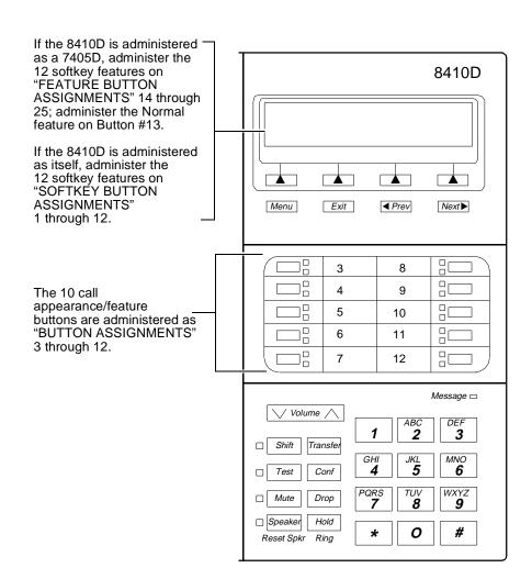
Figure 12-10. Button Numbering for Administering the 8410 Voice Terminal Connected to a System 85 or a DEFINITY G2
