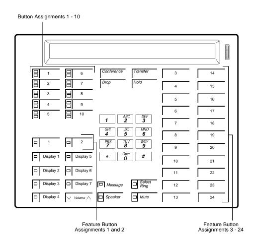
Figure 11-22. Button Numbering for Administering the Enhanced 7407D (7407D02C)
