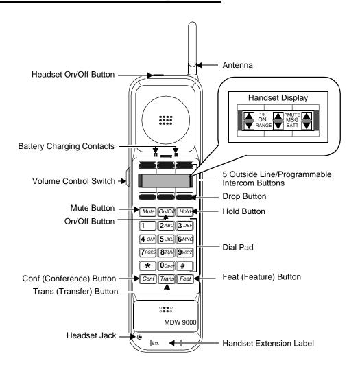
Figure 17-5. The MDW 9000 Telephone, Including Enlarged Display Area
