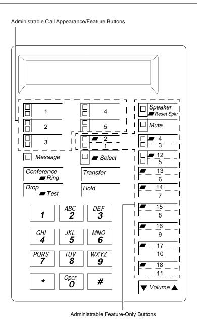
Figure 11-15. Button Numbering for Administering the 7406 Plus Voice Terminal Connected to a System 75, a DEFINITY G1 or G3, or a DEFINITY ECS
