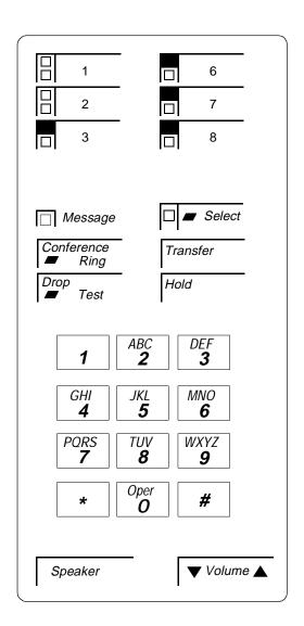
Figure 11-5. Button Numbering for Administering the 7402 Plus Voice Terminal Connected to a System 75, a DEFINITY G1 or G3, or a DEFINITY ECS
