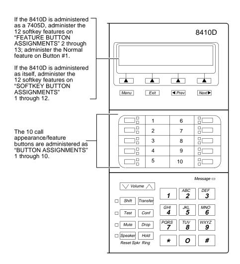
Figure 12-9. Button Numbering for Administering the 8410 Voice Terminal Connected to a System 75, a DEFINITY G1 or G3, or a DEFINITY ECS
