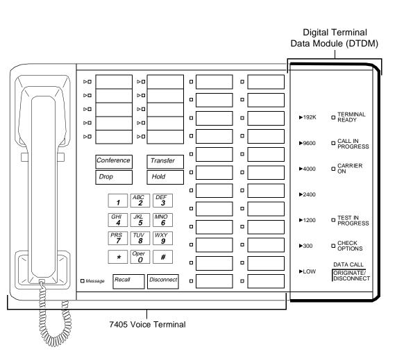
Figure 20-10. The Digital Terminal Data Module mounted on a 7405D Voice Terminal
