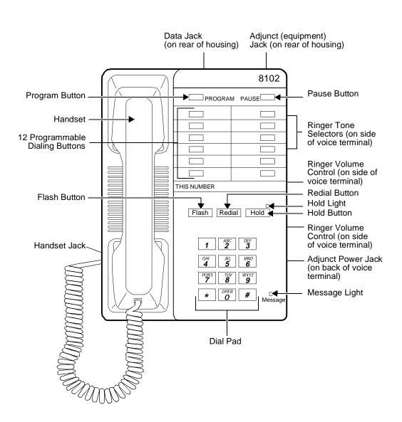
Figure 15-3. The 8102 and 8102M Telephone
