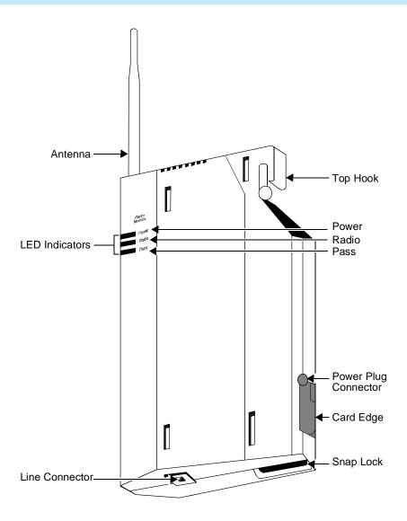
Figure 17-7. The MDW 9000 Telephone, Radio Module
