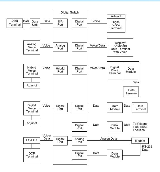
Figure 1-1. Interface Between System Switch and Typical Terminals/Adjuncts
