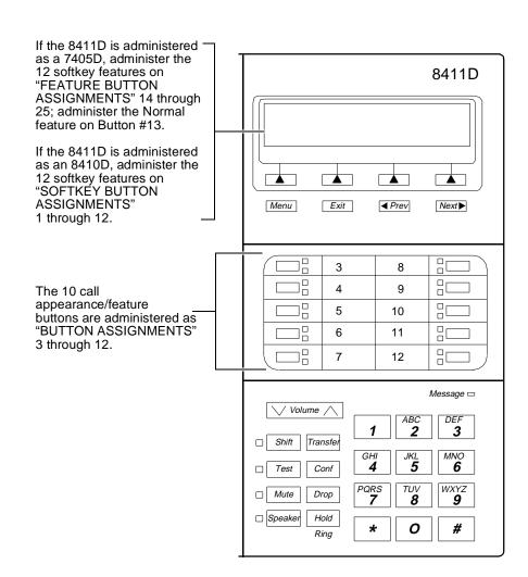
Figure 12-15. Button Numbering for Administering the 8411 Voice Terminal Connected to a System 85 or a DEFINITY G2
