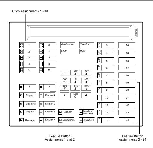
Figure 11-20. Button Numbering for Administering the 7407D (7407D01B)
