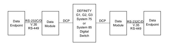
Figure 2-3. Data Link Components
