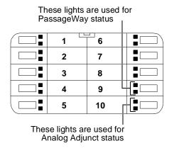
Figure 12-13. The Location of Buttons #9 and #10 on the 8411
