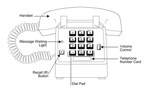
Figure 14-5. The 2500 DMGC Telephone
