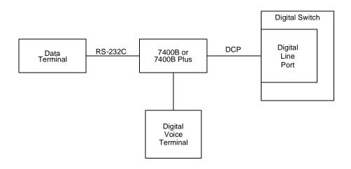
Figure 20-3. A Block Diagram of the 7400B Interface
