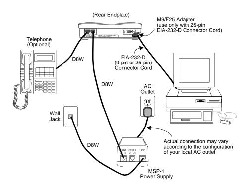
Figure 20-7. Typical Installation of the International Configuration, Including Telephone and Separate Power Supply
