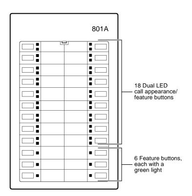
Figure 19-4. The 801A Expansion Module
