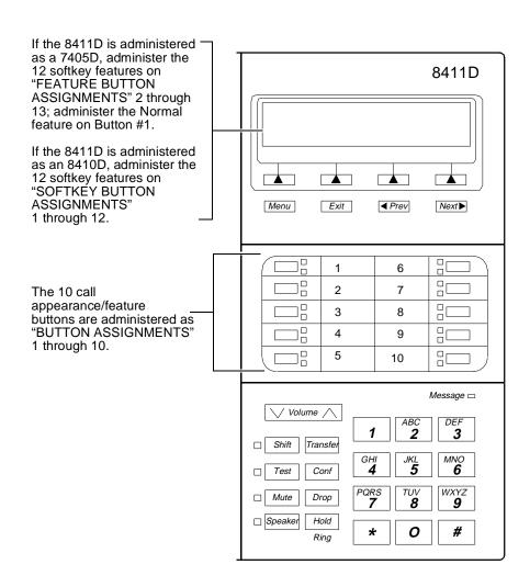
Figure 12-14. Button Numbering for Administering the 8411 Voice Terminal Connected to a System 75, a DEFINITY G1 or G3, or a DEFINITY ECS
