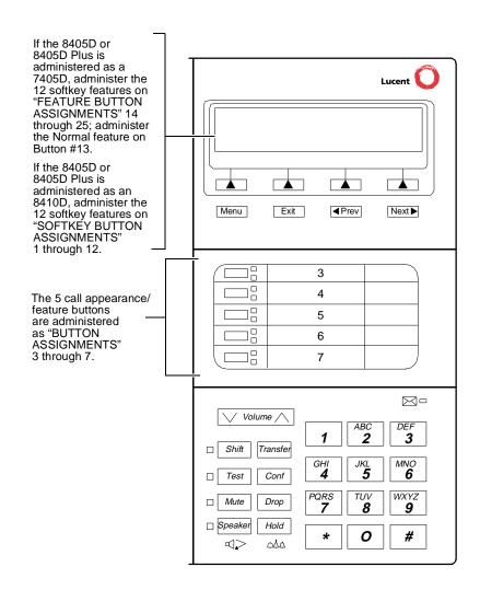
Figure 12-7. Button Numbering for Administering the 8405 Voice Terminal Connected to a System 85 or a DEFINITY G2
