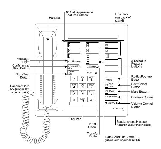
Figure 16-1. The 7505 Asynchronous Data Modular Terminal
