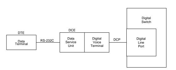
Figure 20-13. A Block Diagram of Z702AL1 Data Service Unit Interfaces
