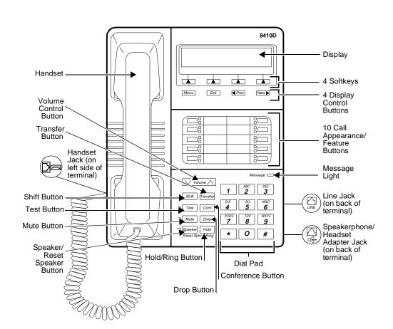
Figure 12-8. The 8410D Voice Terminal (with Display)
