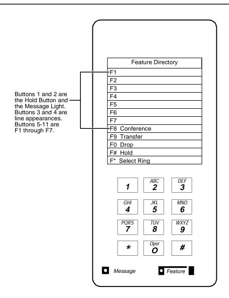
Figure 11-3. Button Numbering for Administering the 7401D and 7401 Plus Voice Terminals Connected to a System 85 or a DEFINITY G2
