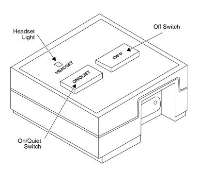
Figure 19-6. The 500A Headset Adapter
