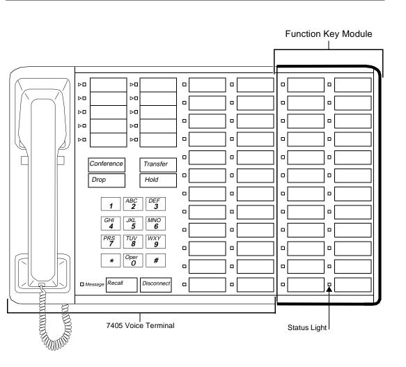
Figure 19-3. The F201 or F401A Function Key Module Mounted on a 7405D Voice Terminal
