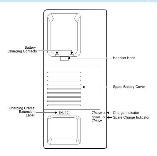
Figure 17-6. The MDW 9000 Telephone, Top View of Charging Cradle
