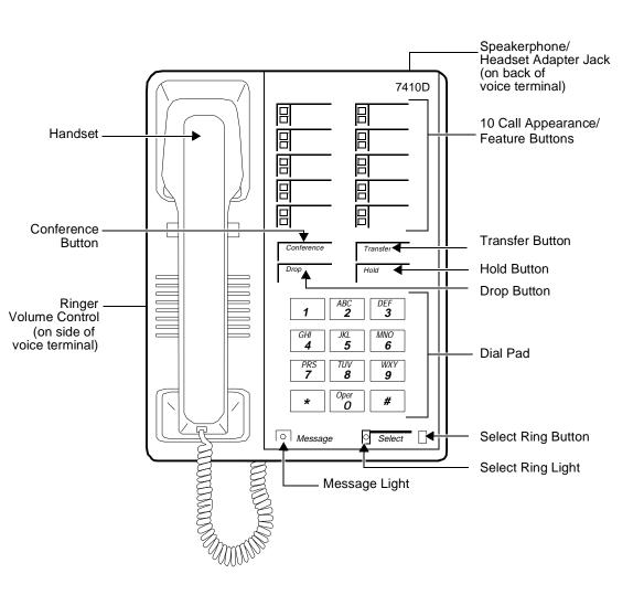
Figure 11-26. The 7410D (7401D01A) Voice Terminal
