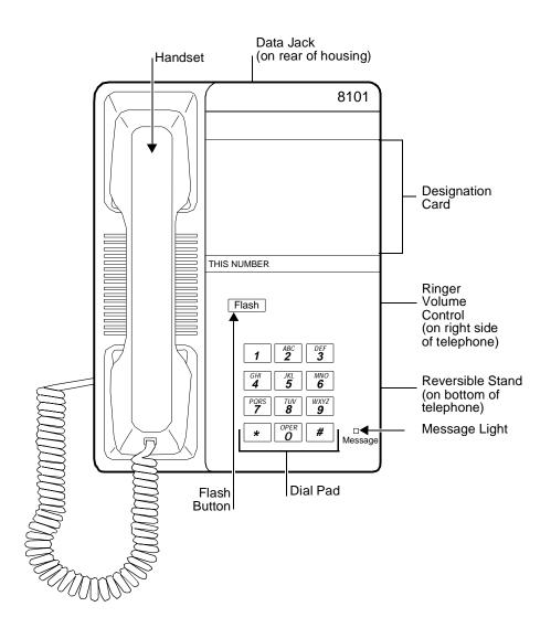
Figure 15-2. The 8101M Telephone
