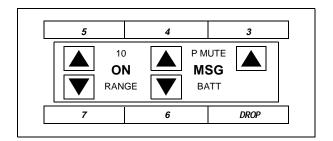
Figure 17-9. Button Numbering for an MDW 9000 Connected to a System 85 or a DEFINITY Generic 2
