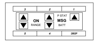
Figure 17-3. Button Numbering for a MDC 9000 Connected to System 75, a DEFINITY Generic 1 or Generic 3, or a DEFINITY ECS
