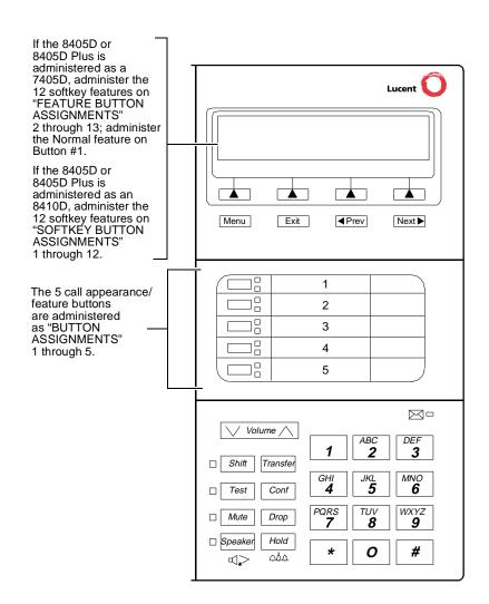
Figure 12-6. Button Numbering for Administering the 8405 Voice Terminal Connected to a System 75, a DEFINITY G1 or G3, or a DEFINITY ECS
