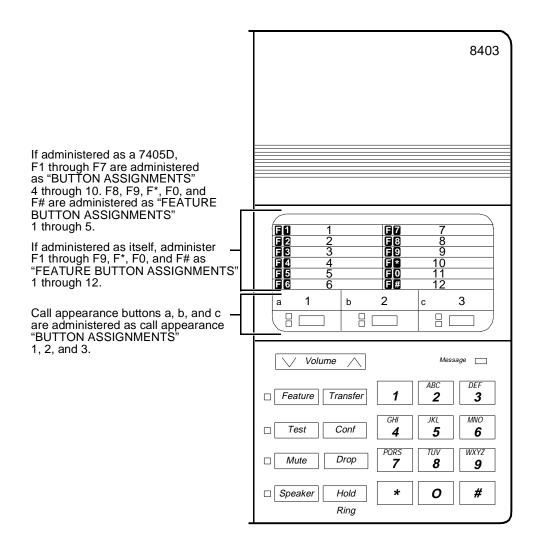
Figure 12-2. Button Numbering for Administering the 8403 Voice Terminal Connected to a System 75, DEFINITY G1 or G3, or DEFINITY ECS
