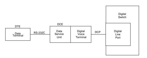
Figure 20-15. A Block Diagram of 703A Data Service Unit Interfaces
