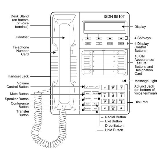
Figure 16-5. The ISDN 8510T Voice/Data Terminal
