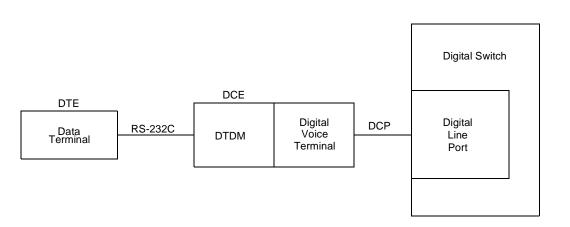
Figure 20-11. A Block Diagram of DTDM Interfaces
