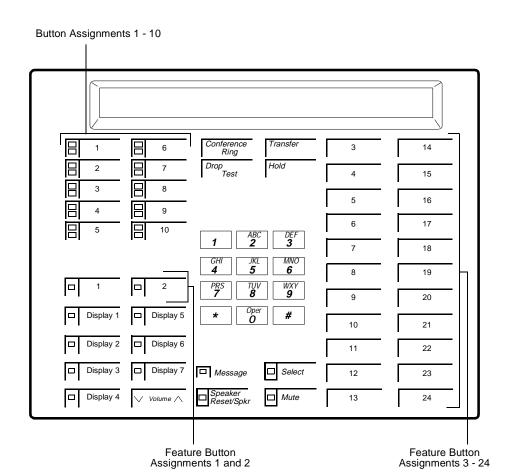
Figure 11-24. Button Numbering for Administering the 7407 Plus Voice Terminal Connected to a System 75, a DEFINITY G1 or G3, or a DEFINITY ECS
