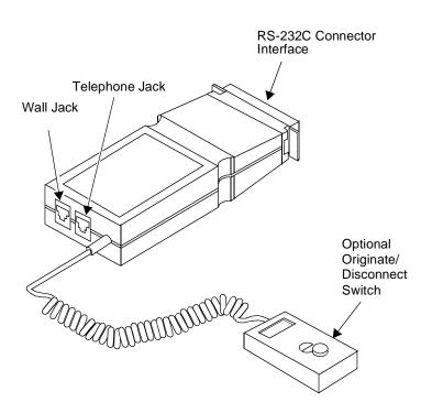
Figure 20-25. The Z3A Asynchronous Data Unit
