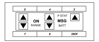
Figure 17-4. Button Numbering for a MDC 9000 Connected to System 85 or a DEFINITY Generic 2
