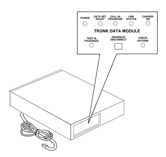
Figure 20-20. The Trunk Data Module, The Stand-alone Model
