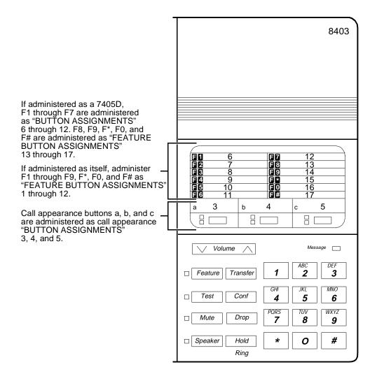
Figure 12-3. Button Numbering for Administering the 8403 Voice Terminal Connected to a System 85 or a DEFINITY G2
