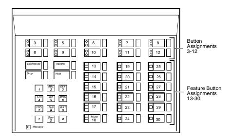
NOTE: The Hold Button is Button #1. The Message Light is Button #2. The Mute Button is Button #18.
