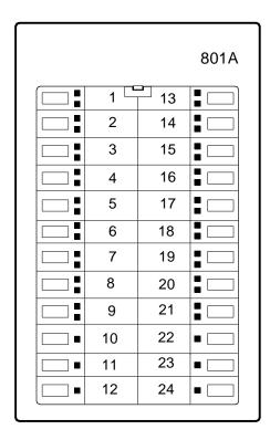
Figure 19-5. Button Numbering for Administering the 801A Expansion Module
