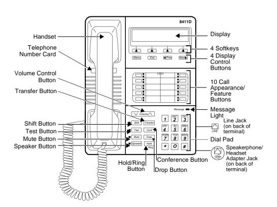
Figure 12-11. The 8411D Voice Terminal (With Display)
