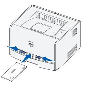
**3** Hold both sides of the print media close to the manual feeder and push it into the printer until it automatically engages.
