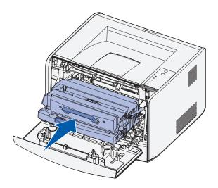
7 After you replace the imaging drum, you should reset the imaging drum's counter. To reset the counter, press and hold the **Cancel** button until all lights flash in sequence.
