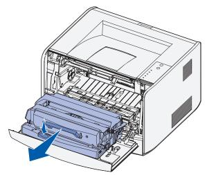
Place the toner cartridge assembly on a flat, clean surface.
