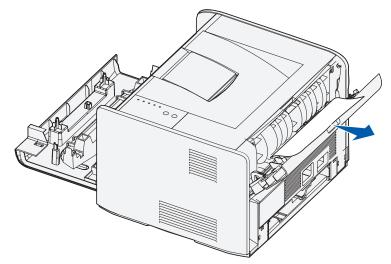
6 After you have cleared the jams, reinstall the toner cartridge assembly, make sure all printer covers and trays are closed, and then press **Continue** to resume printing.
