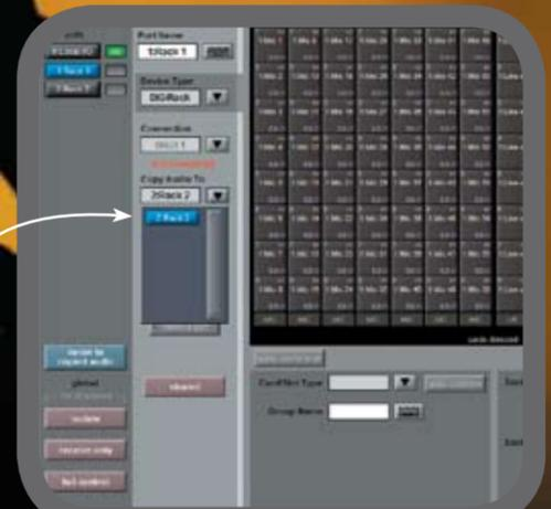
Simple copy to MADi function allowing all remote Mic Pre's to be fed to recording device via console.
