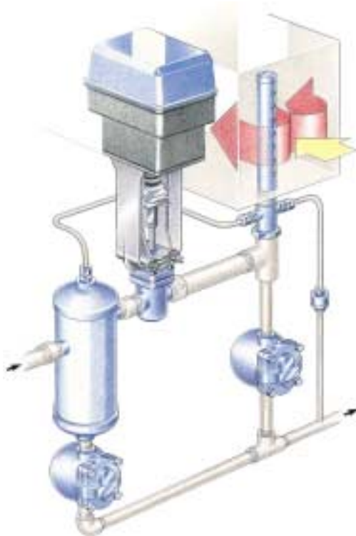
Vertical lance in horizontal duct
