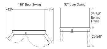
Allow minimum clearances for freezer door and fresh food door for a full 130° door swing and to allow for pan removal.
