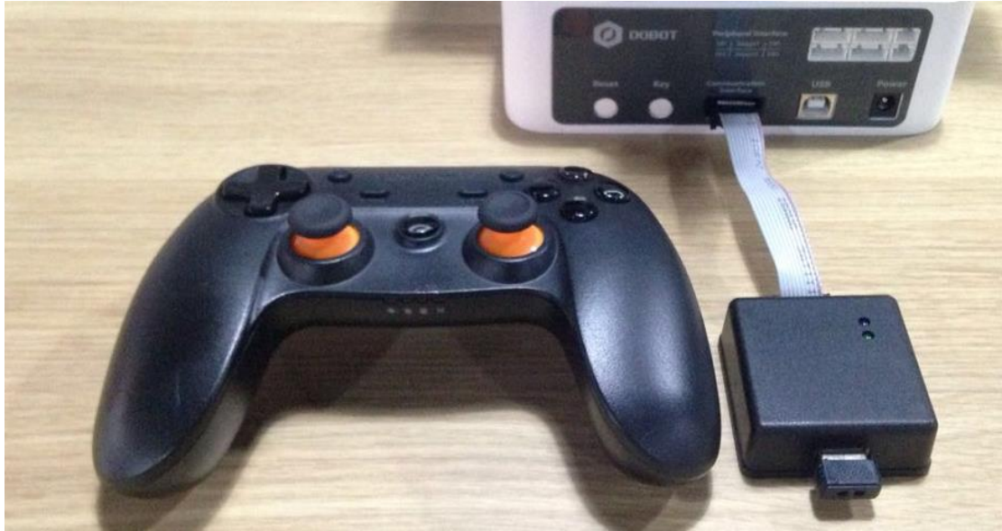
Figure 11.1 Installation of stick module
