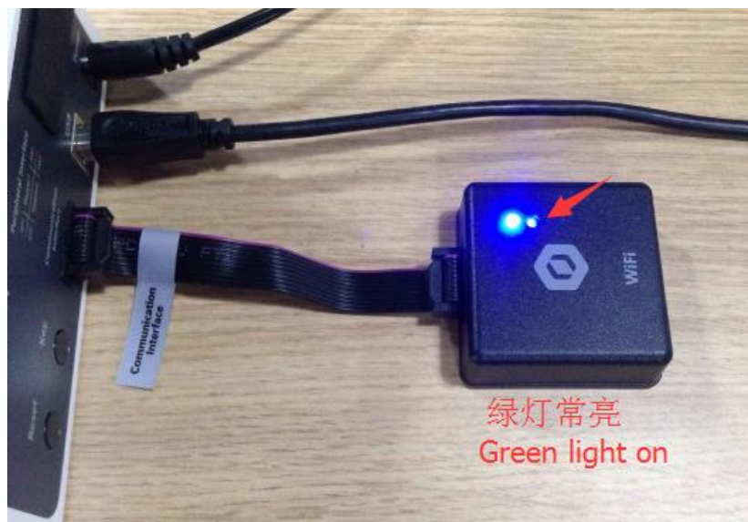
Figure 9.3 Connected with WLAN
