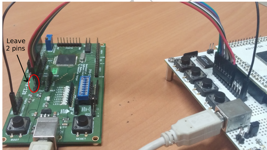
Figure 6.6: Hardware Connection between CPLD and Ptx-128 using 8-PIN Female Connector
