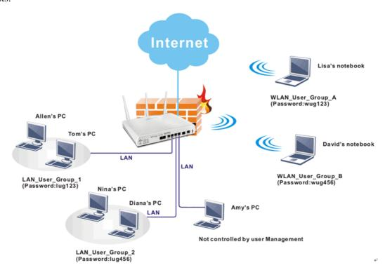
**Note**: Filter rules configured under Firewall usually are applied to the host (the one that the router installed) only. With user management, the rules can be applied to every user connected to the router with customized profiles.
