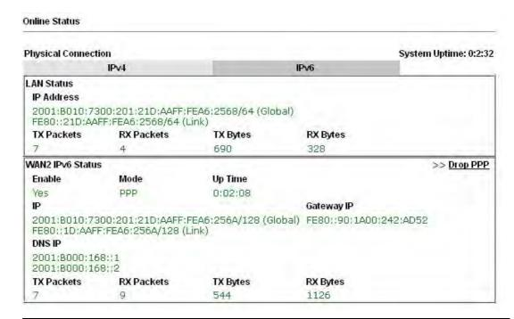
**Note**: At present, the **IPv6 prefix** can be acquired via the PPPoE mode connection which is available for the areas such as Taiwan (hinet), the Netherlands, Australia and UK.
