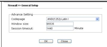
Codepage - This function is used to compare the characters among different languages. Choose correct codepage can help the system obtaining correct ASCII after decoding data from URL and enhance the correctness of URL Content Filter. The default value for this setting is ANSI 1252 Latin I. If you do not choose any codepage, no decoding job of URL will be processed. Please use the drop-down list to choose a codepage.
