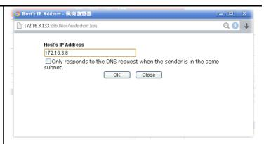
Only responds to the DNS.... – Different LAN PCs can share the same domain name. However, you have to check this box to make the router identify & respond the IP address for the DNS query coming from different LAN PC.
