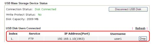
Now, users in LAN of Vigor2132FVn can access into the USB storage device by typing ftp://192.168.1.1 on any browser. They can add or remove files / directories, depending on the Access Rule for FTP account settings in USB Application >> USB User Management.
