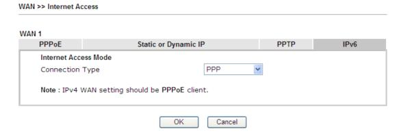
Below shows an example for successful IPv6 connection based on PPP mode.
