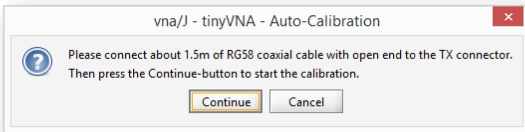
Please attach a RG-58 coaxial cable to the TX connector and click **Continue**. Now four scans are executed. After the fourth scan, a message box is shown, that now the calibration data will be calculated.
