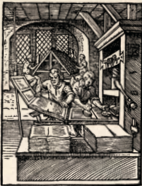
Gutenberg-style printing press from 1568. Such presses could make 240 prints per hour.
