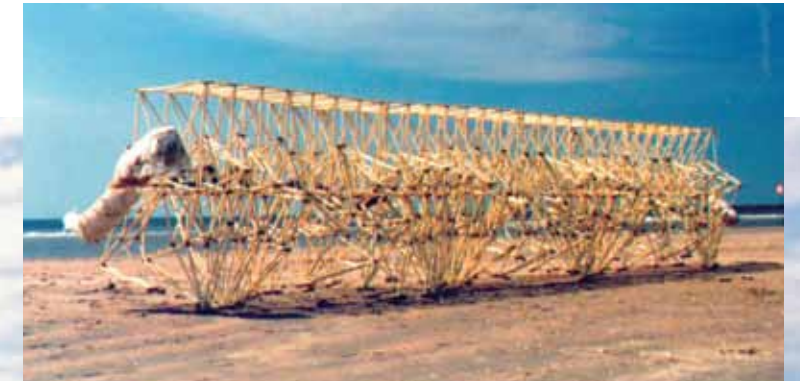
↑ Animaris geneticus ondula Each leg was controlled by a special angled crank so that each leg moves slightly differently. The legs move like a wave in the ocean. 1.7x8.5x2
