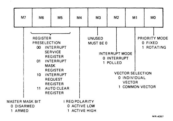
Figure 2-11 Mode Register Bit Assignments
