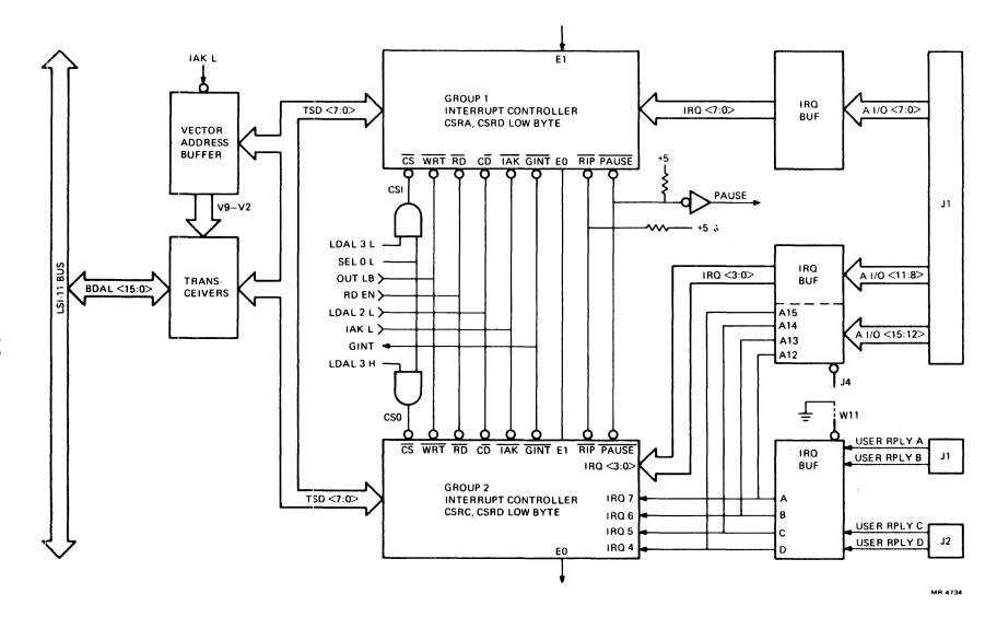
Figure 2-7 Group 1 and Group 2 Interrupt Controller Interconnections
