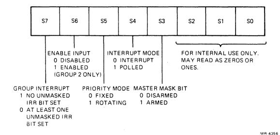
Figure 2-10 CSRA and CSRC Status Registers' Bit Assignments
