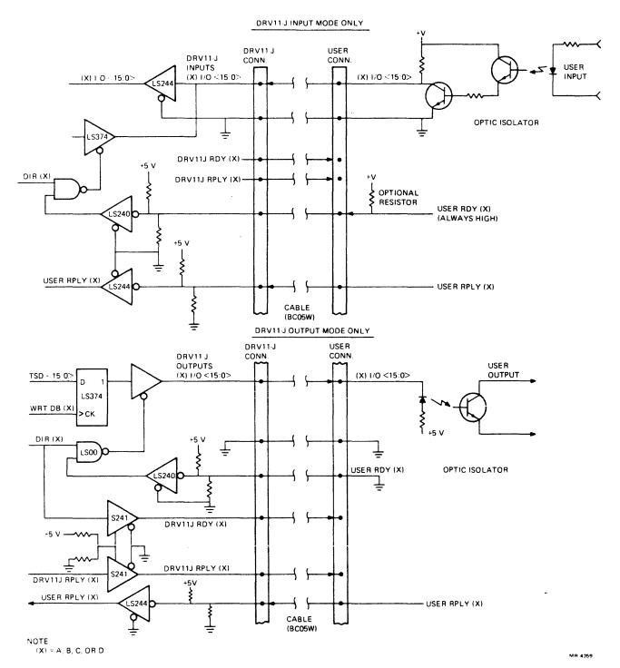
Figure 6-1 Example of an Optic Isolator Interface
