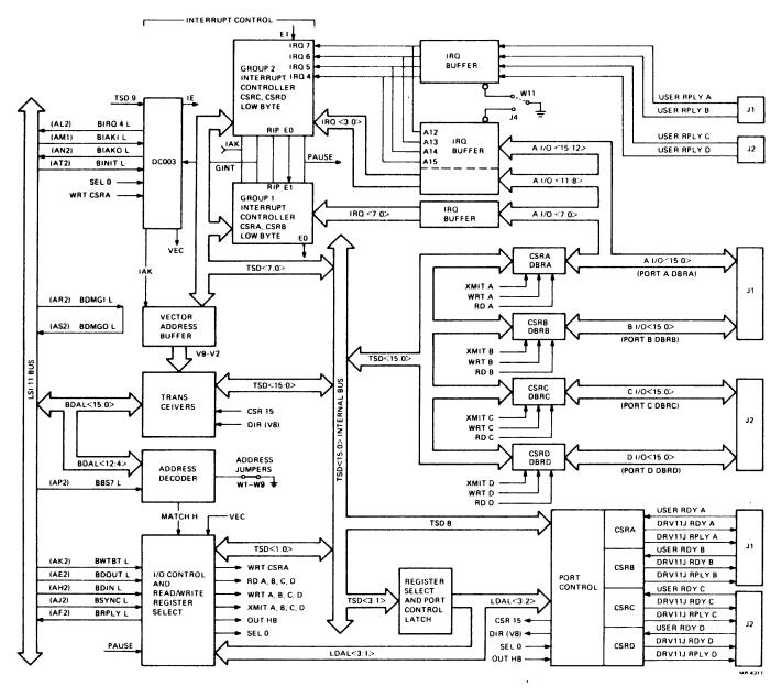
Figure 2-1 DRV11-J Block Diagram
