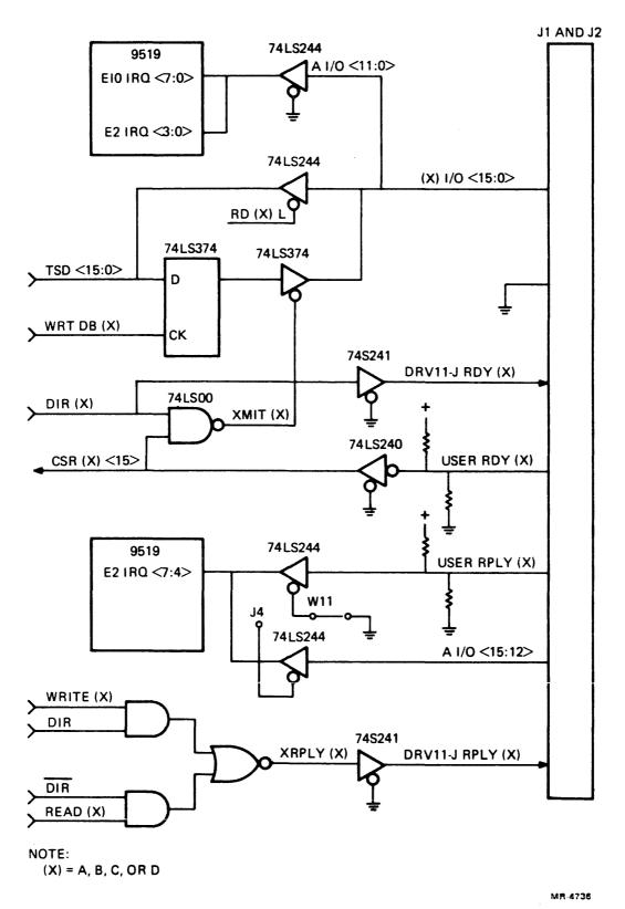
Figure 4-2 I/O Bus Interface, Simplified Schematic
