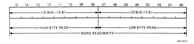
Figure 2-6 Data Buffer Register Bit Assignments
