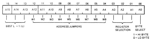
INSTALLED = ALLOWS MATCH TO OCCUR WITH A 1 (LOW) ON THE CORRESPONDING BUS LINE. REMOVED = ALLOWS MATCH TO OCCUR WITH A 0 (HIGH) ON THE CORRESPONDING BUS LINE.
