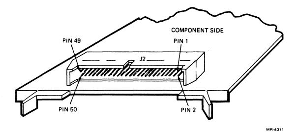
Figure 4-1 DRV11-J I/O Connector Pin Locations
