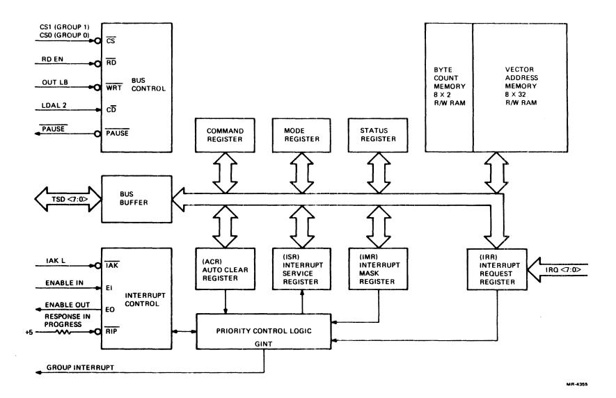
Figure 2-9 Interrupt Controller Block Diagram
