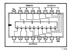
Figure A-1 7442 Package and Logic Diagrams
