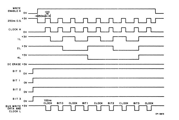
Figure 4-5 Write Clock and Multiplexer Timing Diagram
