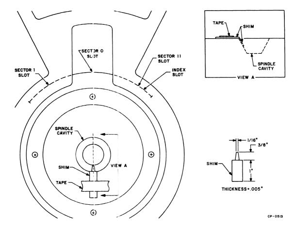
Figure 6-2 CE Test Cartridge Shim Installation
