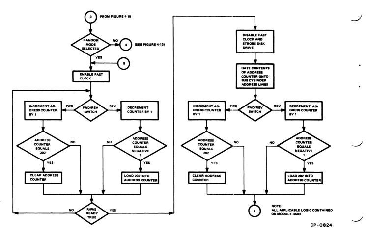
Figure 4-16 Positioner Exerciser Random Mode Flow Diagram
