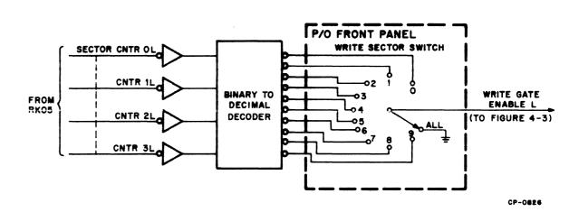
Figure 4-2 Sector Decoder and Write Section Switch Diagram
