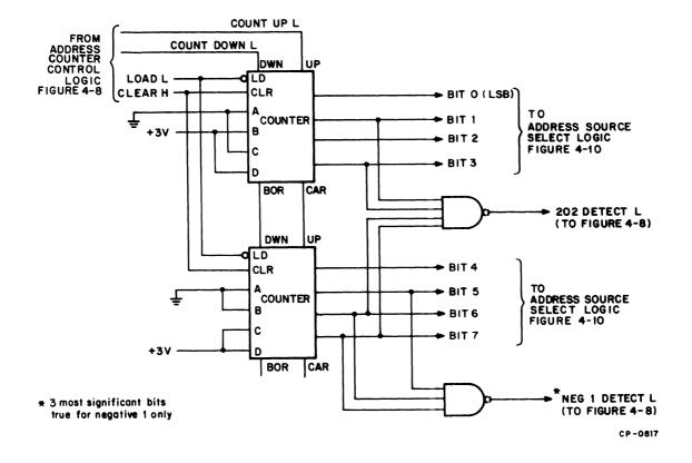
Figure 4-9 Address Counter Logic
