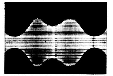
Figure 6-12 2315 CE Pack Head Alignment Waveforms
