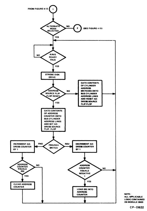
Figure 4-14 Positioner Exerciser Alternate Mode Flow Diagram
