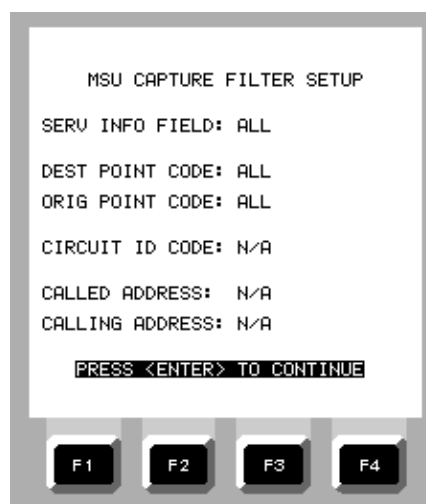
Figure 2-131. SS7 MSU CAPTURE FILTER SETUP Screen
