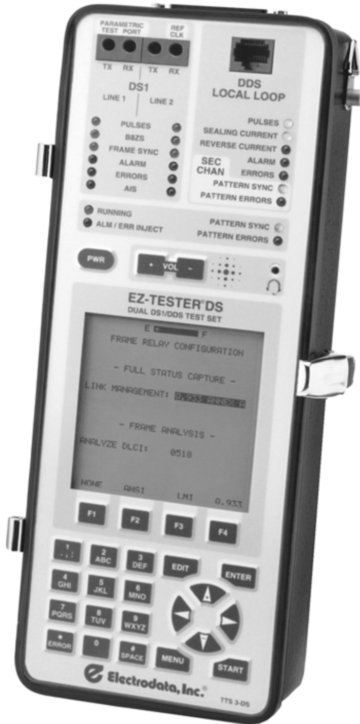
Figure 1-1. EZ-TESTER DS DDS, Dual DS1 Test Set
