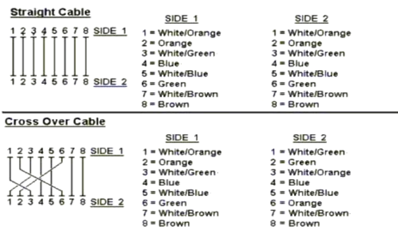
Figure A-1: Straight-Through and Crossover Cable
