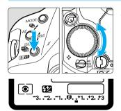
While pressing the <◎⅓> button, turn the <∅> dial to set the desired flash exposure compensation amount.
