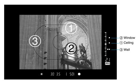
While referring to the exposure level indicator's three spot metering marks, you can set exposure compensation to obtain the desired result.
