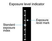
Refer to the exposure level indicator and set the shutter speed and aperture to obtain the desired exposure level.
