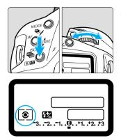
While pressing the <◎∰≥ button, turn the <△⇒ dial until the desired metering mode icon appears.
