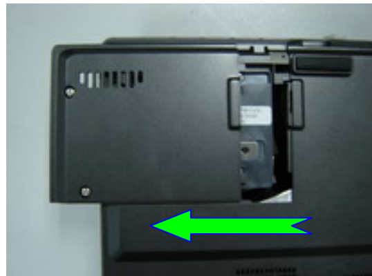
Remove and take out the lamp cover.
