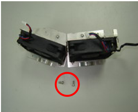
Take off the Fan module and review the screws (S12).
