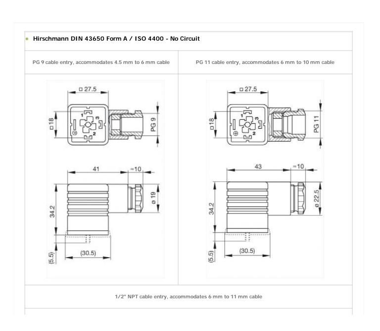
Din 43650 Form A Connector - No Circuit
