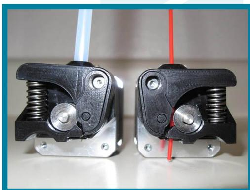
Printrobot Flexible Filament Direct Drive Extruder by thirdhorizon
