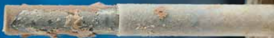
Lime build-up on ordinary probe.
