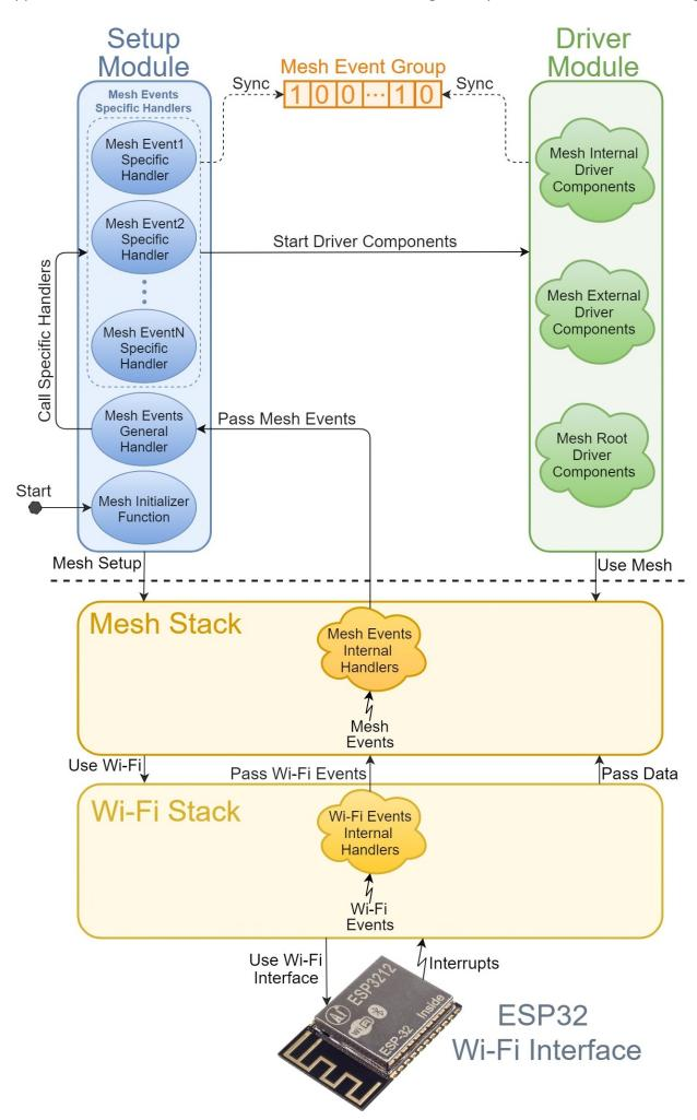
The collection of functions and data structures provided by the ESP-IDF to offer mesh networking functionalities represents the <u>Mesh Stack</u>, which is implemented on top and uses the functionalities offered by the <u>Wi-Fi Stack</u>, which directly manages the device's Wi-Fi interface.
