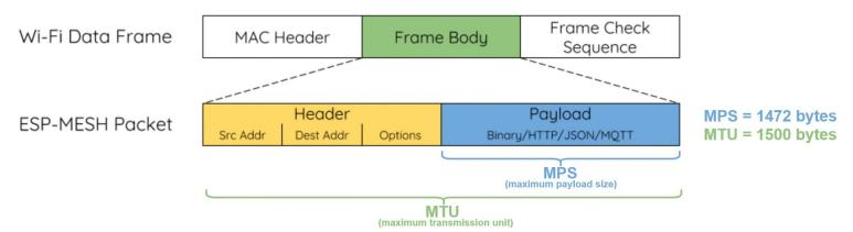
In addition to its payload, which represents the relevant information exchanged between nodes, a mesh packet is comprised of the following information:
