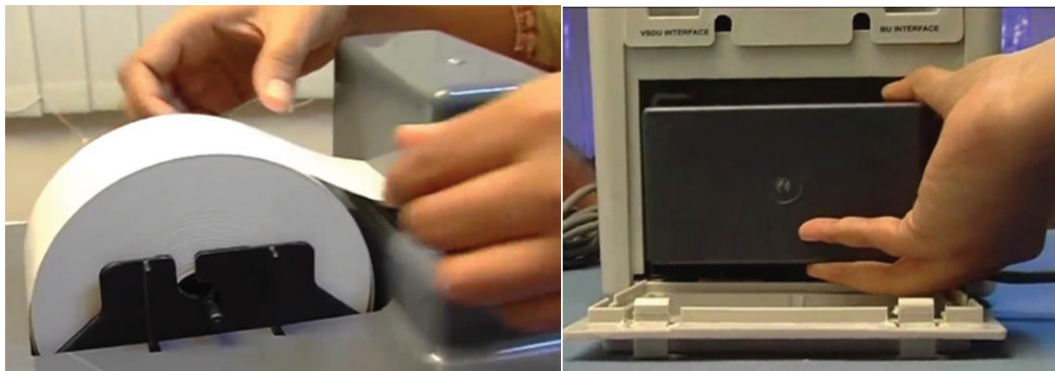
Installation of paper roll
