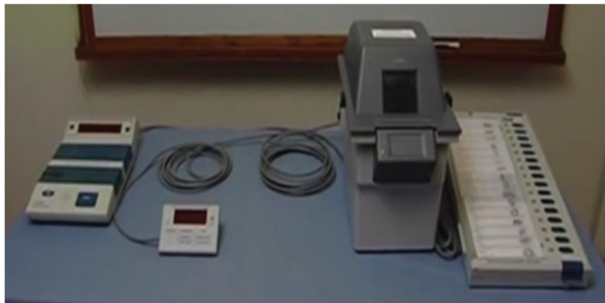
Control Unit VSDU Printer (VVPAT) Balloting Unit
