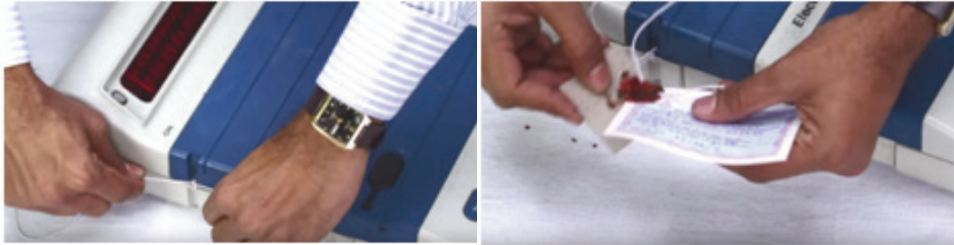
Sealing of outer cover of Candidate Set Section
