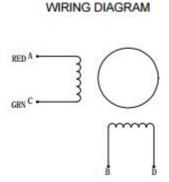
Coil wire diagram from the datasheet our NEMA 16 Stepper Motor with Cable.
