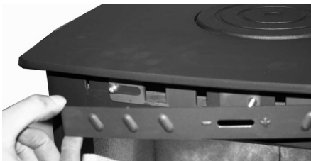
Fig. 15. Lifting cover from body
