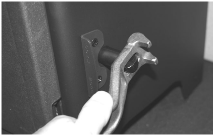
Fig. 24 Setting The Grate
