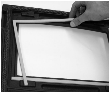
Fig. 17. Lining up the gasket
