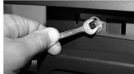
Fig. 16. Inner slider removal
