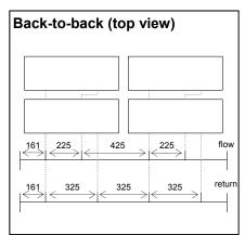
For line configurations of more than 3 boilers and back to back configurations of more than 6 boilers, two collectors have to be connected.
