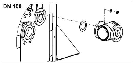
If required by the situation, an extension pipe (optional) can be used to move the location of the gas filter a bit further from the cascade system.
