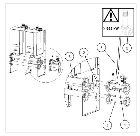
Assemble the ISPESL gas valve to the gas connection as shown in the pictures.
