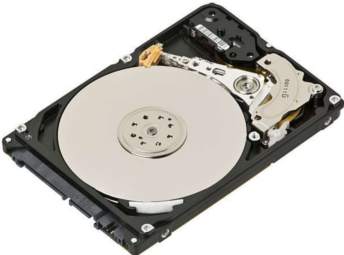
Figure 8-2. A standard 2.5" hard drive, found in most laptops. Source: Wikimedia
