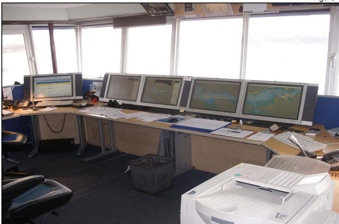
Milford Haven's VTS - photograph showing the 4 screens displaying radar pictures
