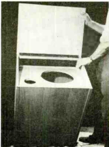
Enclosure with speaker board in position.
