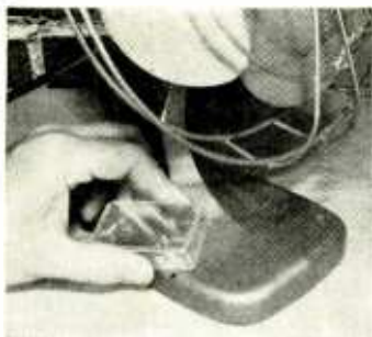
High-impedance pickup at right consists of phono cartridge mounted in plastic case. Above, unit is shown detecting vibration in fan base.
