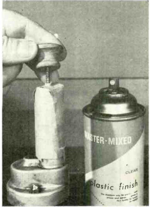
5 Any rotary device, such as the electric drill shown here, can be a big help in spraying small parts evenly.
