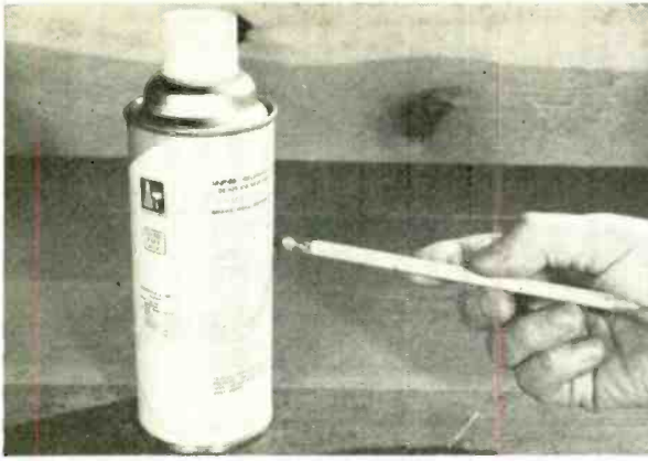
4 An accessory spray head (below) produces a "splatter-type" finish for old cabinets, enclosures, panels.
