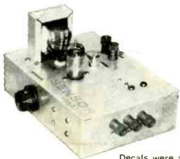
Decals were added to completed relay to identify binding posts and controls.
