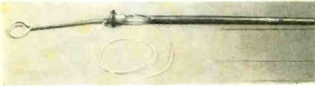
Thermistor can be mounted either in a modified oil dip stick (above) for measuring oil temperature, or in a simple housing (below) for monitoring temperature of cylinder head. See text for details.
