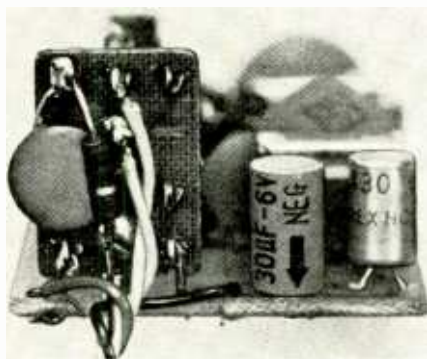
Flexible wire connected between the external components and relay board will prevent breakage due to vibration. Shock-mount unit with foam rubber.
