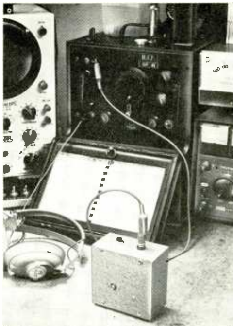
Where accurate frequency check points are a must, as when checking a BC-221 at 100-kc. points, the super calibrator speeds and eases the operation.
