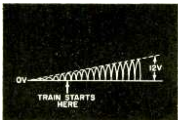
Fig. 1. The ordinary power pack is nothing more than a full-wave rectifier whose output is a pulsating d.c. voltage with peaks that look like the waveform above. For most locos, the average power required for starting is much too high for a smooth start, and the trains pull out with a sudden jerk, and at a speed not akin to real railroading.
