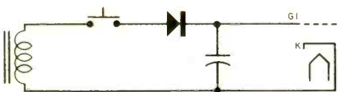
Fig. 4. Momentary application of a high d.c. potential across the cathode and G1 can boost emission.
