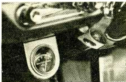
This illuminated voltmeter is one of several types for use in cars. Panel meters will also serve; in some cars, they can be mounted in dash. Meter above is sold by Lafayette Radio.
