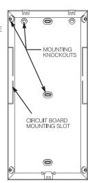
With the circuit board removed, use a small screwdriver to punch out the wiring and mounting knockouts located in the detector's back. Feed the wiring through the wiring knockout and secure the detector to the wall.
